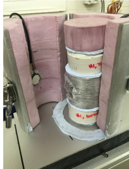
Figure 9 - Current Testing States (a) Sorption samples conditioning at 50% relative humidity (b) Sample labeling convention cut and cored LGCC sample (c) LGCC Test Setup.
