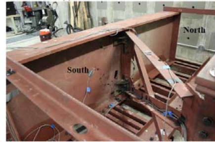
Fig. 4. Test setup of the reduced-scale bridge girder subassemblage model
