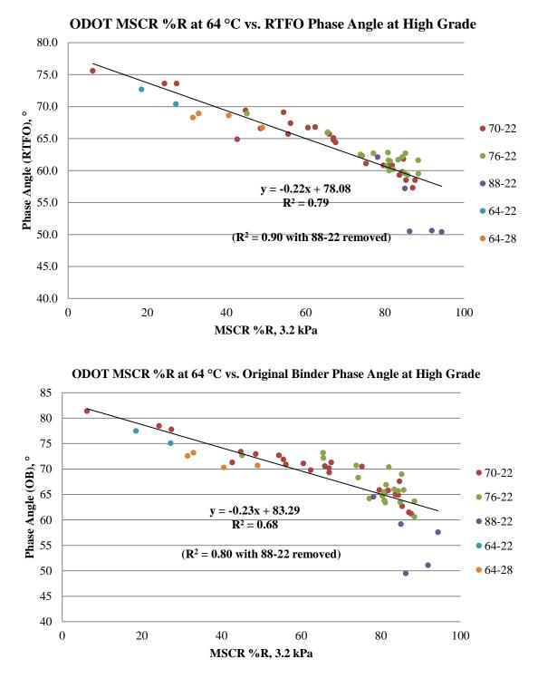
Figure 5. ODOT MSCR %R at 64 C vs. Phase Angle at grade temperature.
