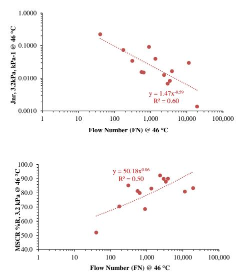
Figure 9. Flow Number testing relative to MSCR data on WCTG mixtures (From [5]).
