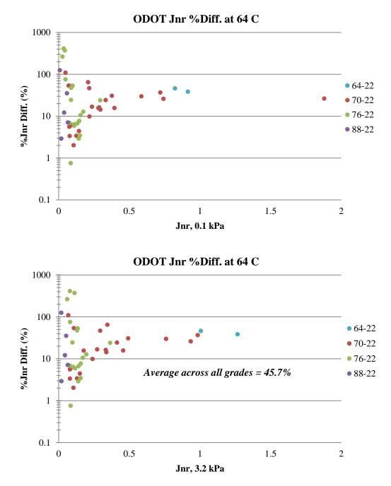
Figure 11. ODOT MSCR %Jnr Diff. vs. Jnr at two stress levels.
