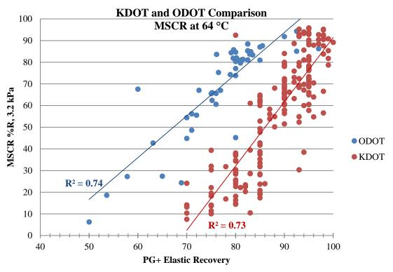
Figure 4. Comparison of KDOT and ODOT data showing effect of PG+ elasticity method.
