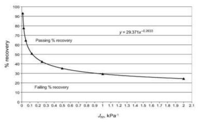
Figure 2. Indication of elastomeric modification, from AASHTO M332-14 [3].
