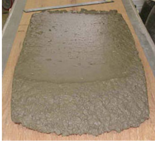
Figure 2. SF SCC pavement slab produced using mini-paver
