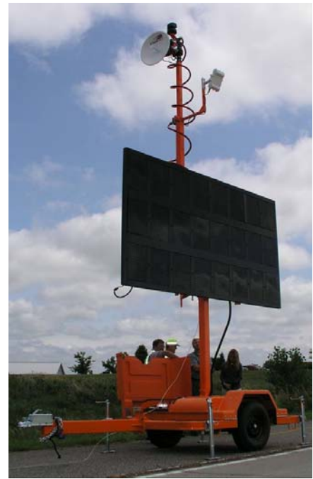
Figure 2.6: Mobile Traffic Surveillance System
