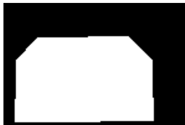
Figure 3.9: A common gusset plate shape for connecting 5 truss members (2 diagonals, 1 vertical, and 2 chord members)
