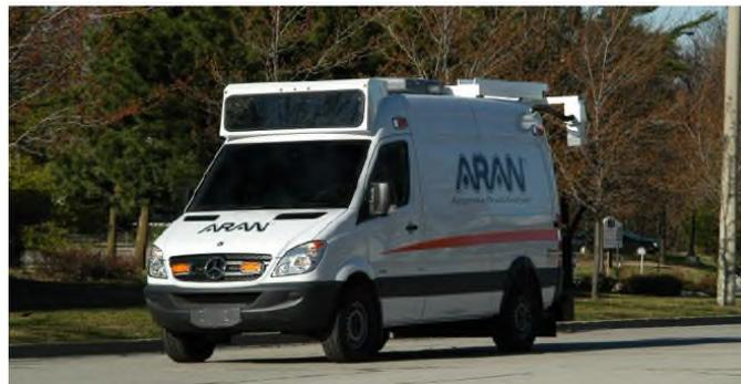
Figure 2.13. Fugro-Roadware multi-function data collection equipment.
