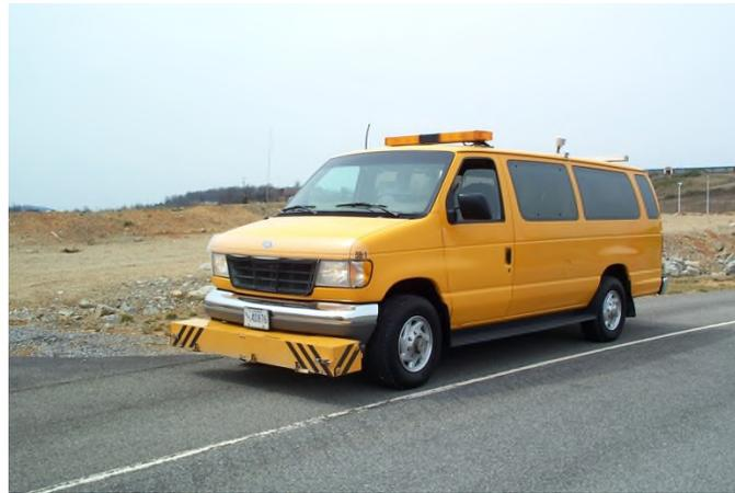
Figure 2.2. High-speed profiler.
