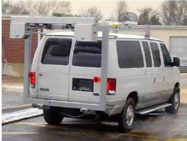
Figure 2.12. Dynatest multi-function data collection equipment.
