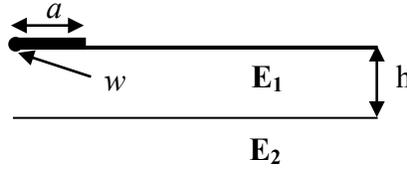
Figure 2- Two-layer system of subgrade with modulus  $E_1$  overlain by base with modulus  $E_2$
