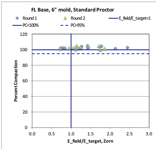
Figure 4- Zorn LWD field surface modulus to the target surface modulus ratio versus percent compaction
