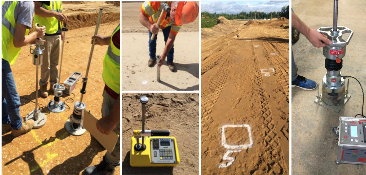
**FIGURE 1 From left to right: LWD testing in the field; NDG testing and MC sample collection; field stations locations; LWD testing on 6” Proctor mold in lab**
