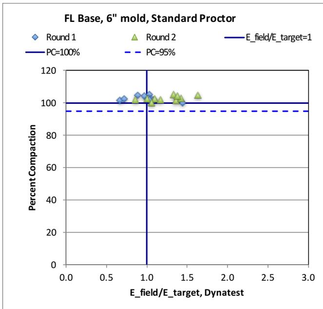
Figure 6- Dynatest LWD field surface modulus to the target surface modulus ratio versus percent compaction
