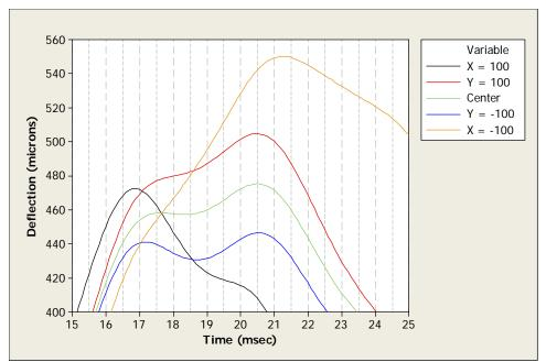
Figure 4 Time histories of 5 geophones on the platter due to one drop.
