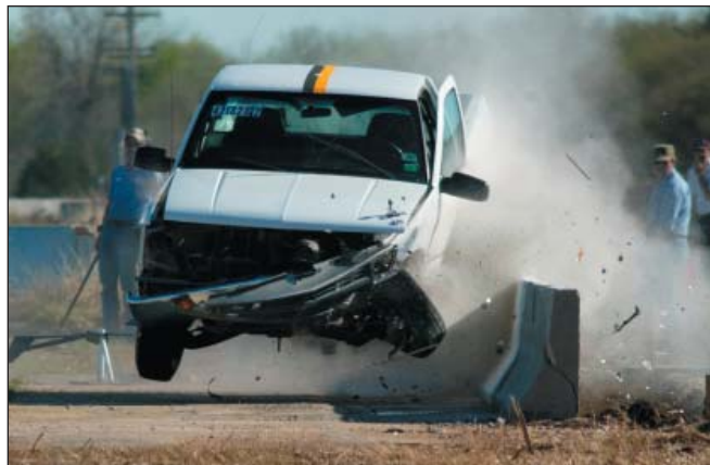
Figure 2. NCHRP Report 350 test 4-11 on the 32-inch (813 mm) Jersey-shaped railing design used in Florida.
