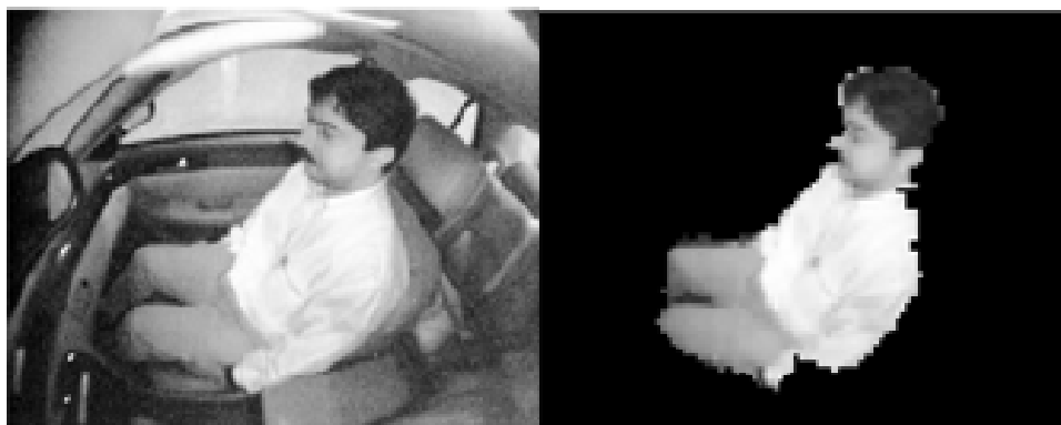
Figure 9. Raw Image (Left) and Extracted Image (Right) of Passenger [24]
