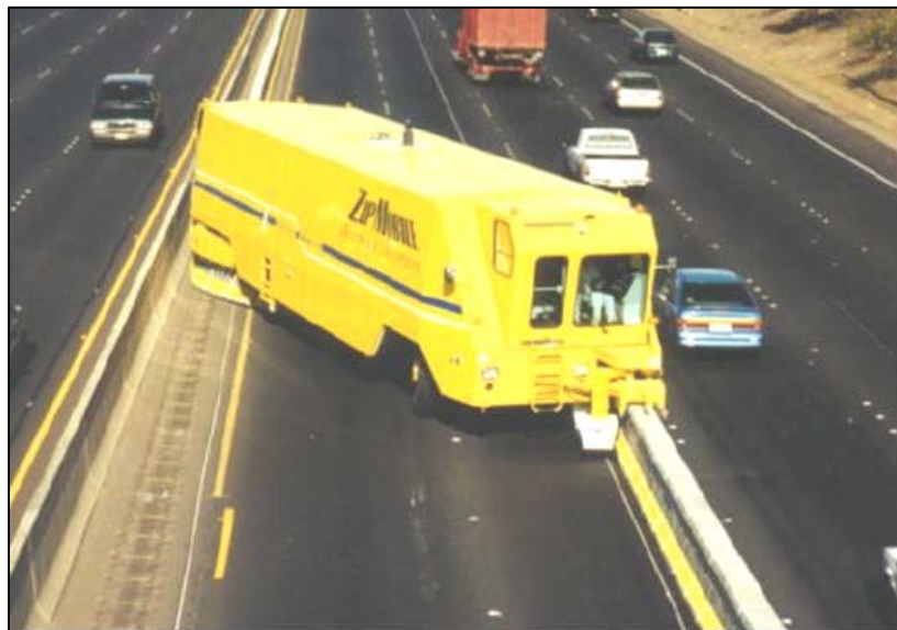
Figure 5-2. Creation of a Barrier-Separated Contraflow Lane by a Zipper Truck 32
