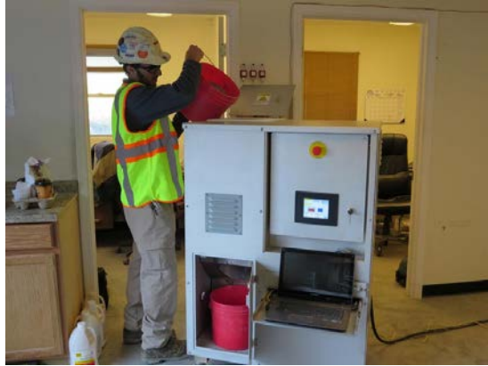
FIGURE 2 Operator feeding aggregate sample into enclosed SLT cabinet.
