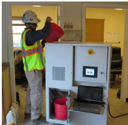
FIGURE 1 Operator pouring aggregate sample into SLT Laser Scanning System.
