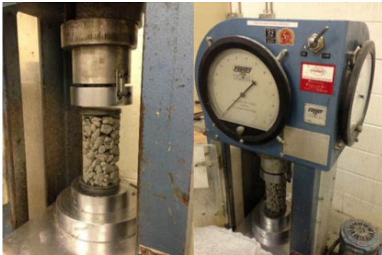
Figure 13. Capped CTPB Specimen Loaded for Compressive Strength Testing.
