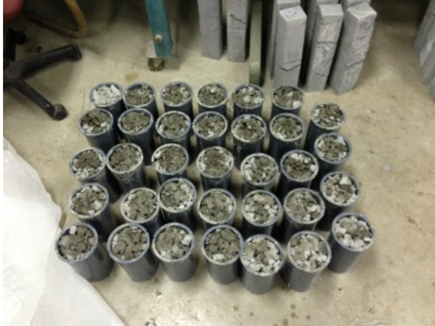
Figure 2. Fabricated CTPB Specimens from Oklahoma.
