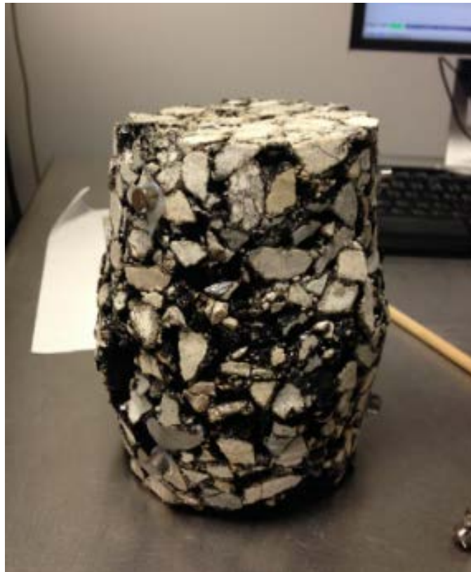
Figure 6. Plastically Deformed ATPB Specimen During Dynamic Modulus Testing at High Stress Levels and High Temperatures.
