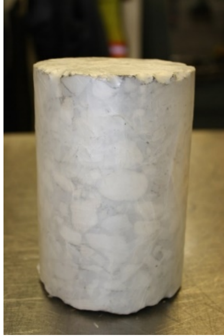
Figure 3a. Specimen Wrapped in Parafilm.
