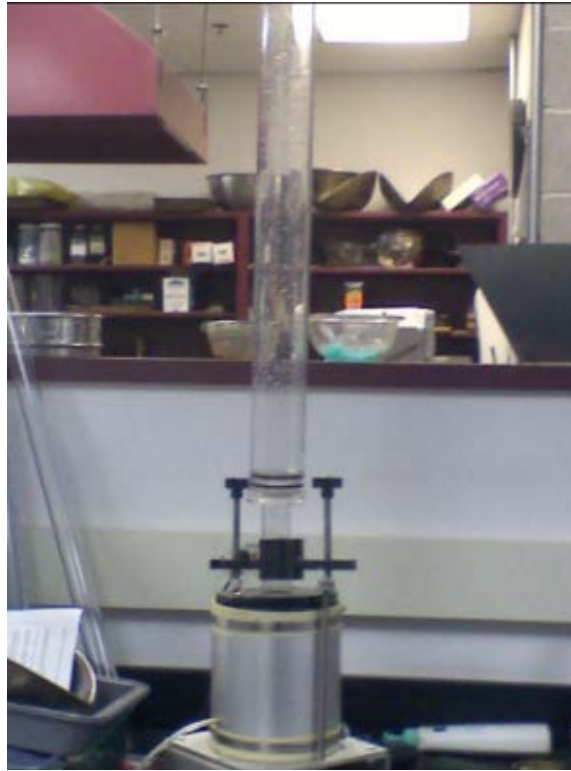
Figure 5. Customized Permeameter to Determine Permeability of ATPB Specimens.
