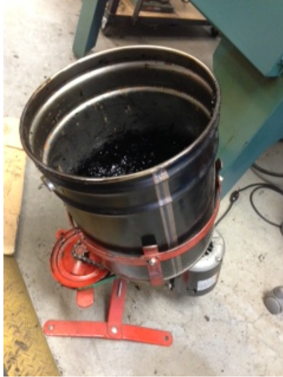
Figure 1. Asphalt Treated Permeable Base from Idaho Fabricated Using a Bucket Mixer.
