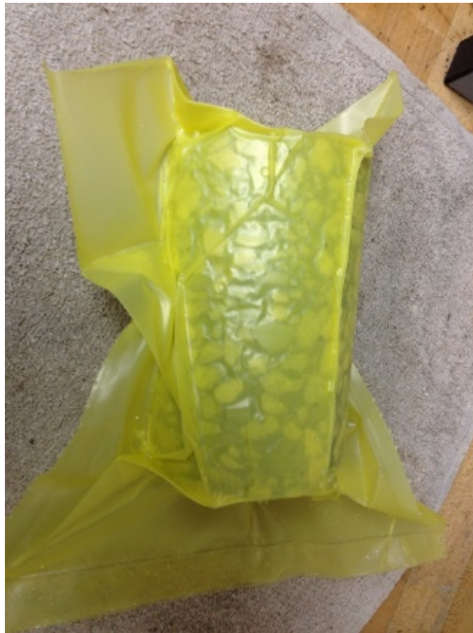
Figure 3b. Specimen Vacuum Sealed.
