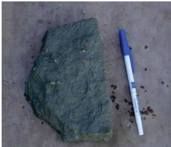
Figure 6.17 An aggregate particle found during placement of LC-HPC 11
