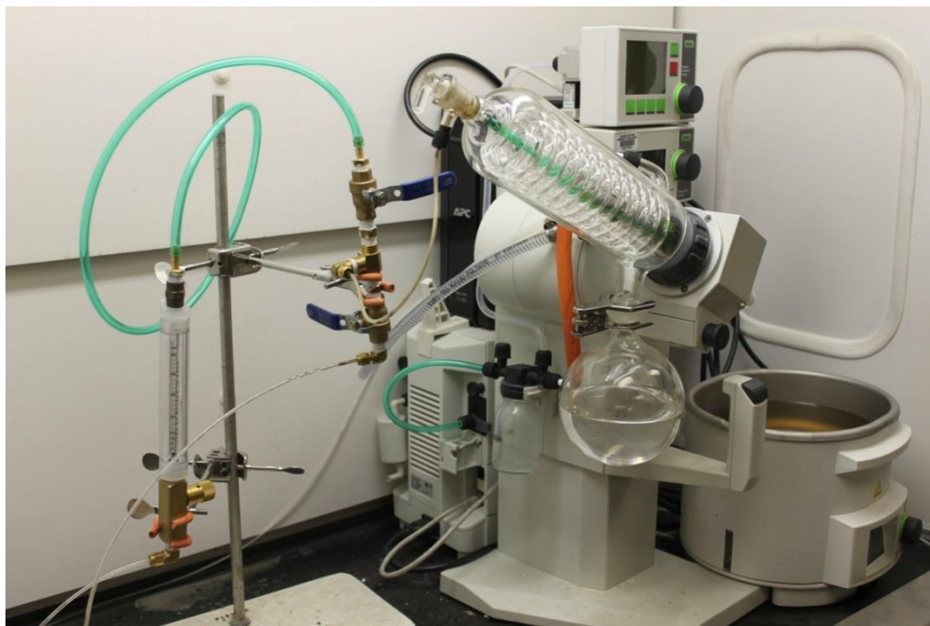
Figure 2.1 Rotatory evaporator system at Rutgers University for asphalt binder recovery
