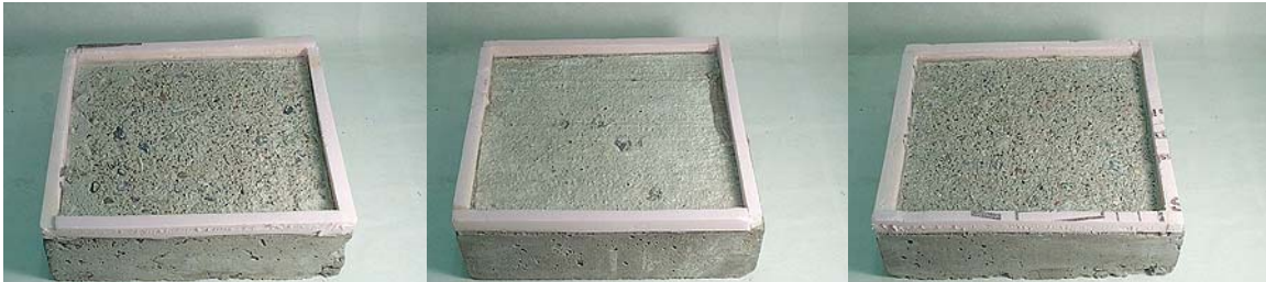
Figure 30: Prisms representative of the five different solutions after 56 days of ASTM C 672 testing.
