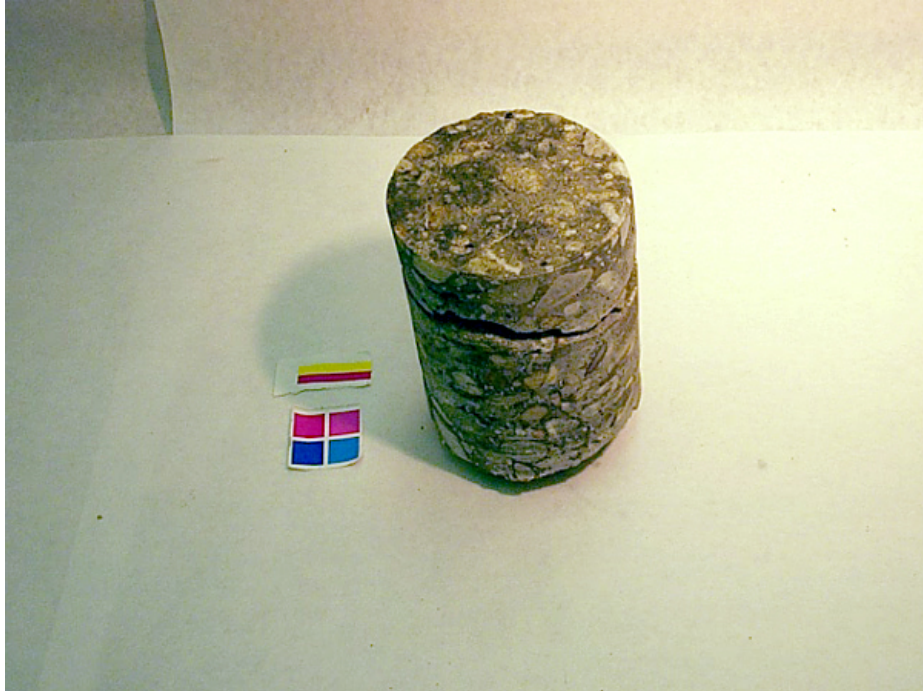
Figure 3: Core T-1, taken adjacent to deteriorated area.
