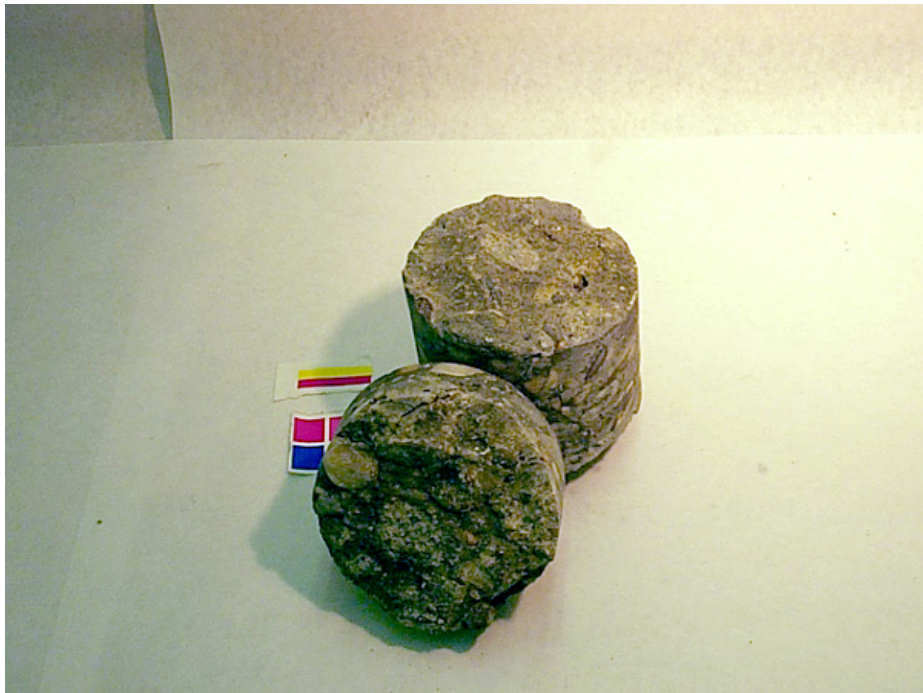
Figure 4: Core T-1, separated to illustrate crack plane.
