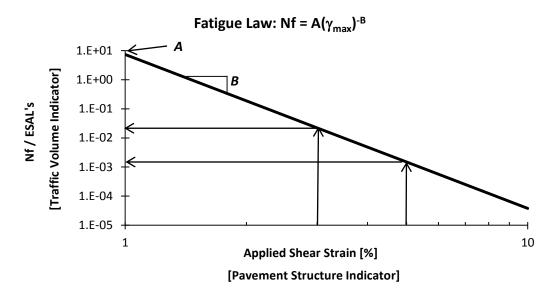
**FIGURE X2.2** – Plot of fatigue parameter  $N_f$  (normalized to 1 million ESAL's) versus applied binder shear strain on a log-log scale. Allowable fatigue life can be determined for given strain amplitudes, as shown by the arrows.
