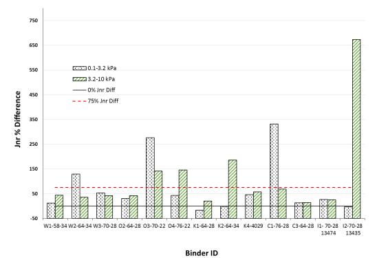
Figure 7. % Jnr Diff values for each Pooled Fund binder. Where 0.1-3.2 kPa data represents the % Jnr Diff between stress levels of 0.1 and 3.2 and 3.2-10 kPa data represents the % Jnr Diff between stress levels of 3.2 and 10 kPa.
