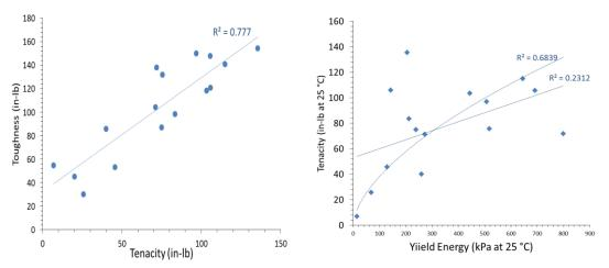
Figure 13. Toughness and tenacity for WCTG samples (left); Tenacity and yield energy at 25 °C (right)
