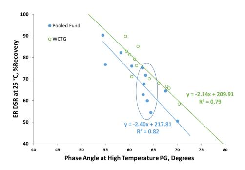
Figure 1. Correlation between Phase Angle and ER DSR results for the Pooled Fund and WCTG data sets.
