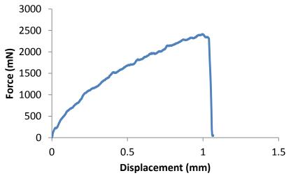
Figure 8.1. Graph. BBR-SENB typical force-displacement curve
