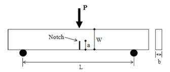
Figure 18. Schematic of SENB testing apparatus. Where P is the point load on the opposite side of the notch [10].
