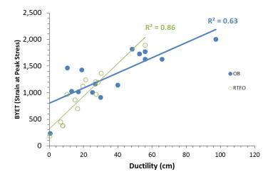
Figure 10. Comparison of BYET Strain at Peak Stress with Ductility at 4 °C.
