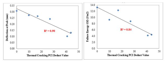
Figure 19. Correlation between deflection at peak load (left) and failure energy (right) with thermal cracking PCI deduct [8].
