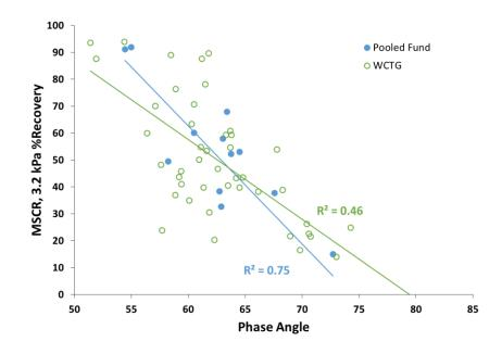
Figure 3. Correlation between Phase Angle and MSCR %R for asphalt binders tested as part of the Pooled Fund and WCTG.
