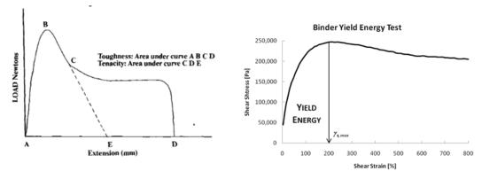
Figure 11. Definition of toughness, tenacity, and yield energy.
