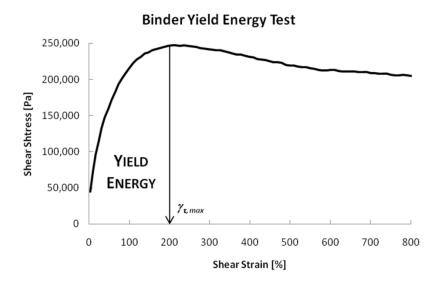
Figure 8. Typical output for BYET test
