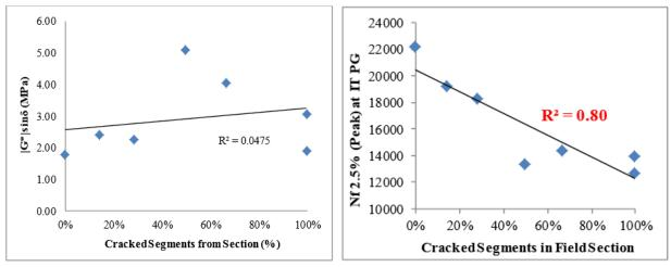
Figure 15. Comparison of Cycles to Failure Measured by LAS test to field fatigue cracking in Wisconsin [8].
