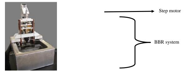
Figure 6.2. Photograph. Loading device in BBR-SENB
