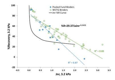
Figure 6. Elastomeric indication chart per AASHTO 332 with current data
