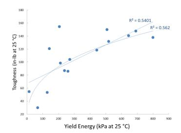
Figure 12. Toughness and Yield Energy at 25 °C for WCTG binder set.
