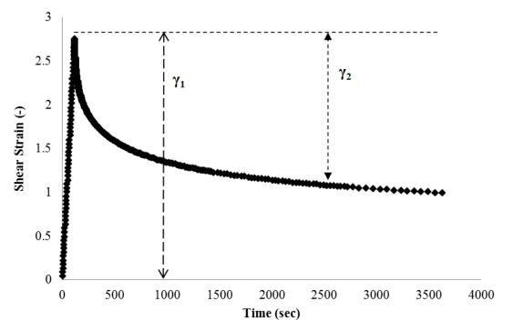
FIGURE 7.2 – Typical  $\gamma(t)$  curve for the elastic recovery test in the DSR
