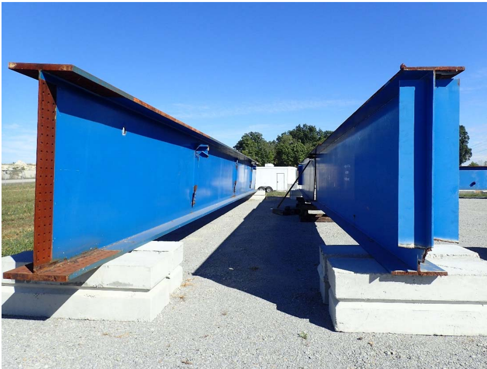
Large plate girders from the Virginia Ave Bridge in Indianapolis
