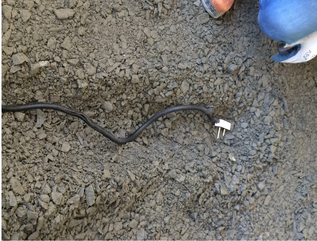
Figure 0.11. Placement of GS-1 VWC sensor in VA21a aggregate
