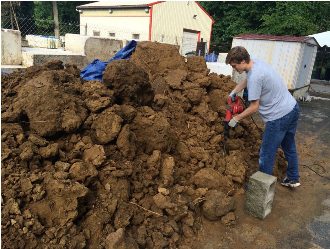
Figure 0.7. Use of hammer jack in breaking the large chunks of HPC soil.
