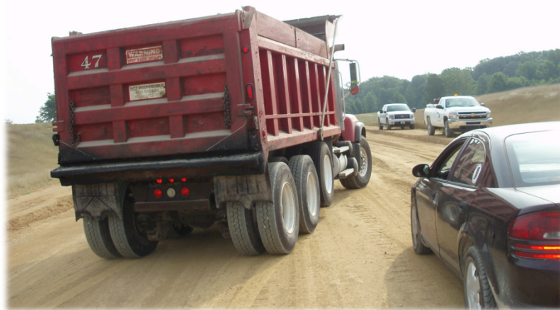
A fully legally loaded tri-axle dump truck. ( About 70,000 lbs.)
