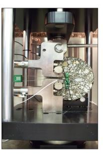
Researchers evaluated core samples from test sites for their resistance to cracking using the disk-shaped compact tension test in which a specimen is loaded to failure.
