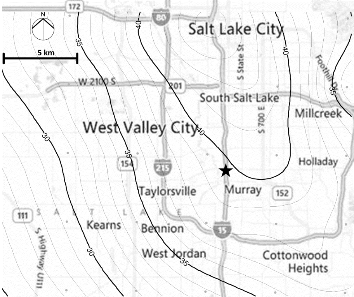
Figure 2-3. Liquefaction loading map ( T_R = 1,033 years) showing contours of CSR^{ref} (%) for a portion of the Salt Lake Valley in Utah.
