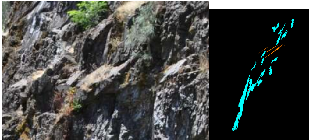
Figure 22. Left is an image of possible planar failure surfaces of approximately 50-degree dipping Joint Set 2 (light orange) with respect to the general rock face, while right shows a side view of Split-FX image of Joint Set 2 (orange) as compared to the main slope surface (teal).
