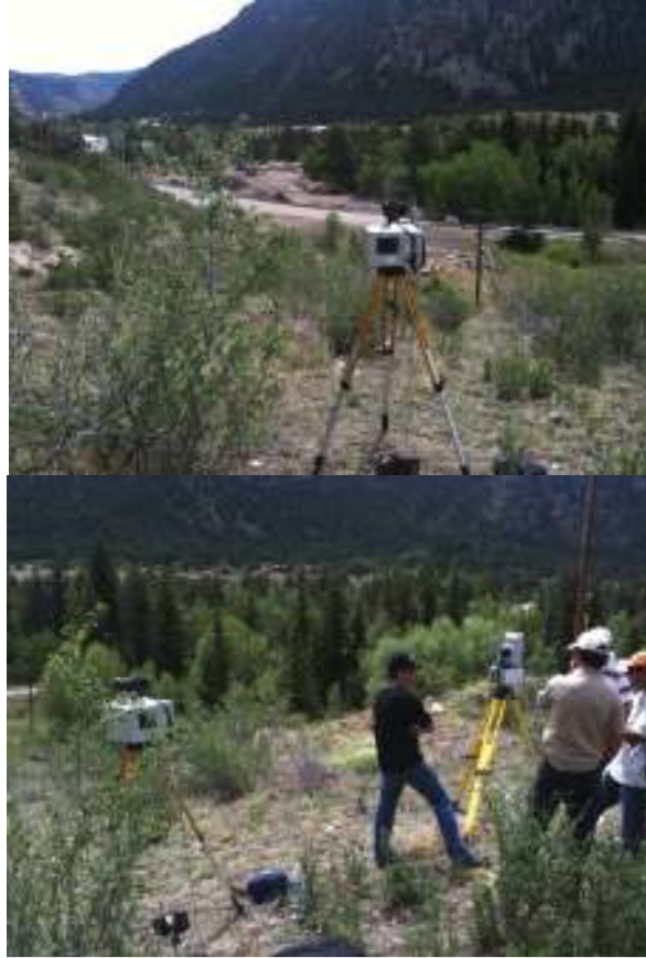
Figure 27b. At Site 2, (top) the Optech scanning of the site from the distance of 286 meters (938 ft), and (bottom) the Optech and ISITE scanners, also at the 286-meter distance.
