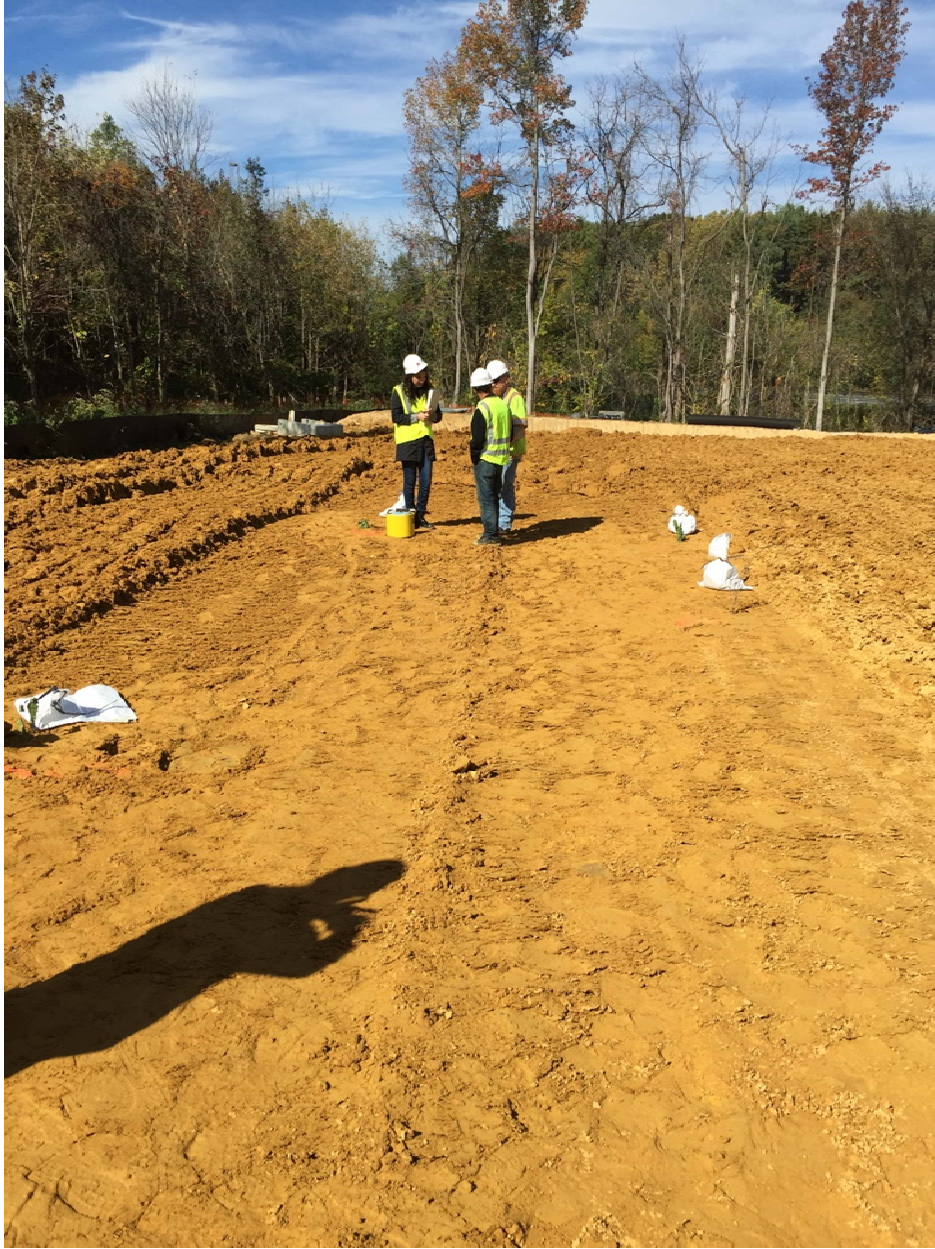
Figure 23. Section 1-4: SM (Silty Sand)
