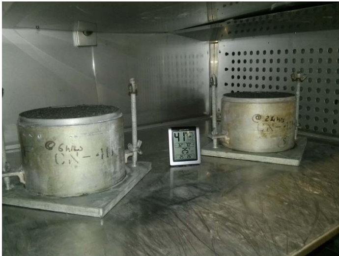
Figure 4 - Drying simulation in the environmental chamber.
