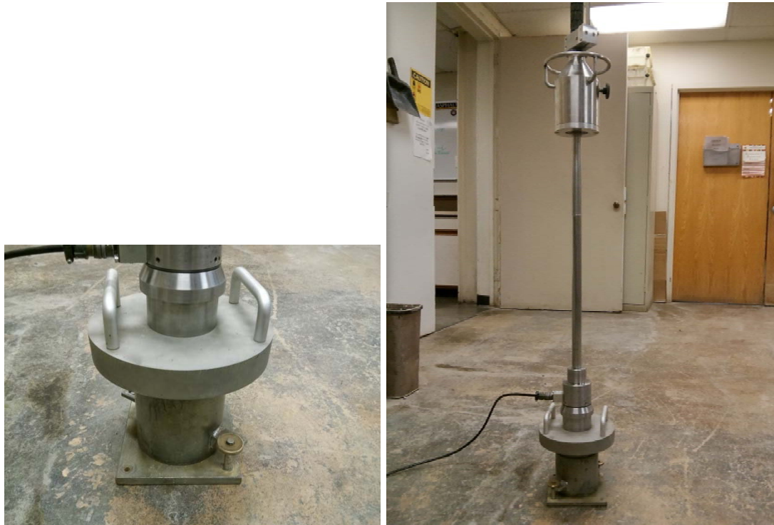
Figure 3 Configuration of Olson LWD test on top of the Proctor mold.
