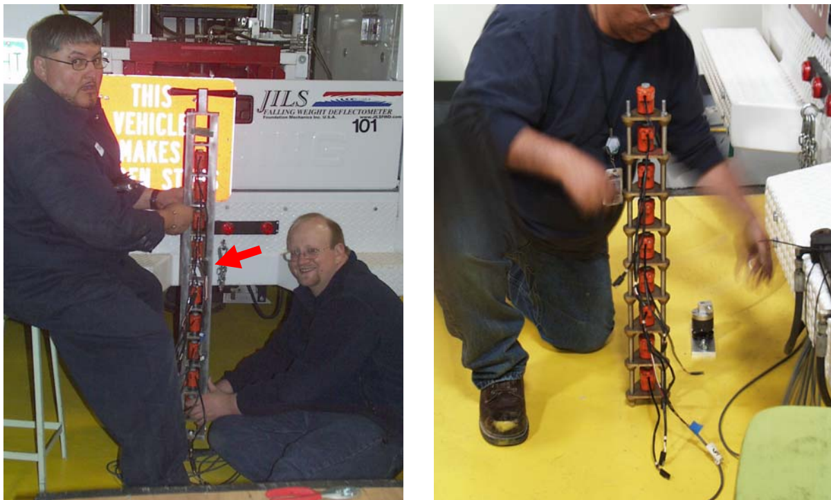
Figure 3. Calibration of the JILS FWD in Denver, CO. Prototype geophone stand on the left, with accelerometer in place (red arrow) for a reference calibration. The same stand is also used for relative calibration. On the right, JILS geophones are stacked in the factory relative calibration stand for comparison of results to the new stand.
