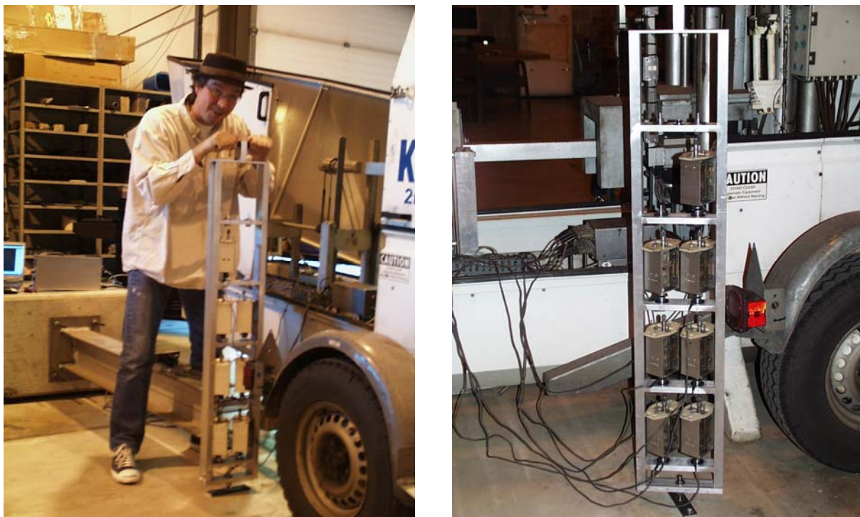
Figure 1. Calibration of KUAB FWD in Harrisburg, PA. The KUAB seismometers were stacked two to a shelf (right).
