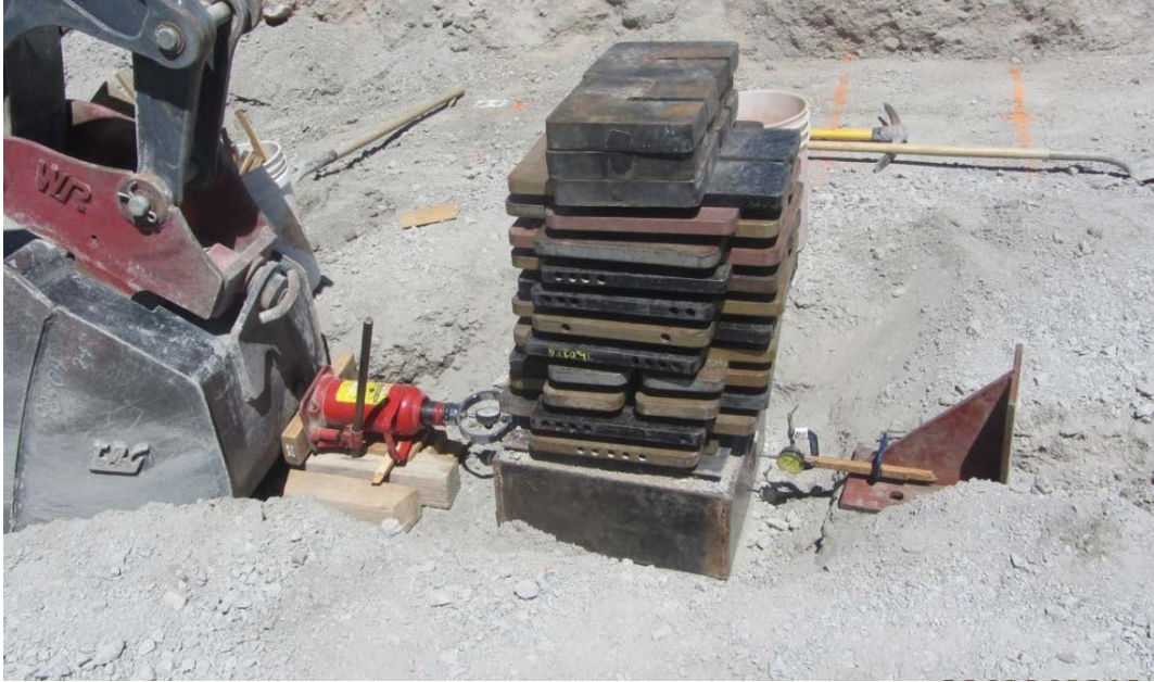
Figure 11. Photo of in-situ direct shear test on gravel backfill
