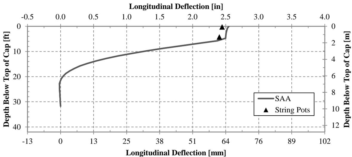
Figure 16. North 5.5-ft backfill 30° skew final deflection comparing shape array and string potentiometers
