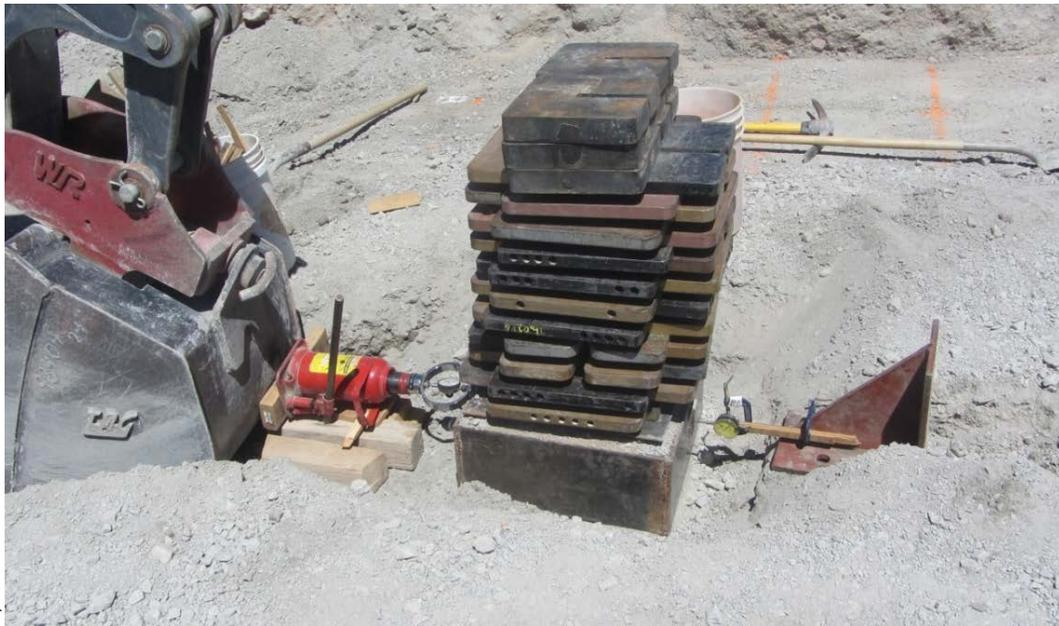
**Figure 10. In situ box direct shear test on gravel backfill**
