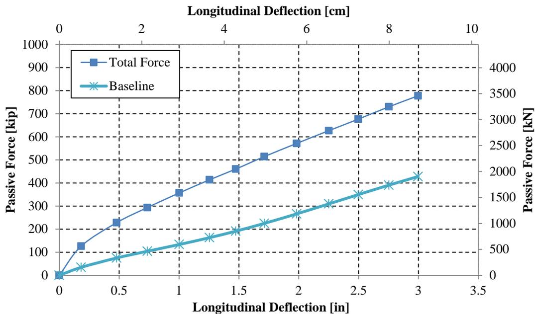
**Figure 12. Total force and baseline resistance for 0° skew test.**
