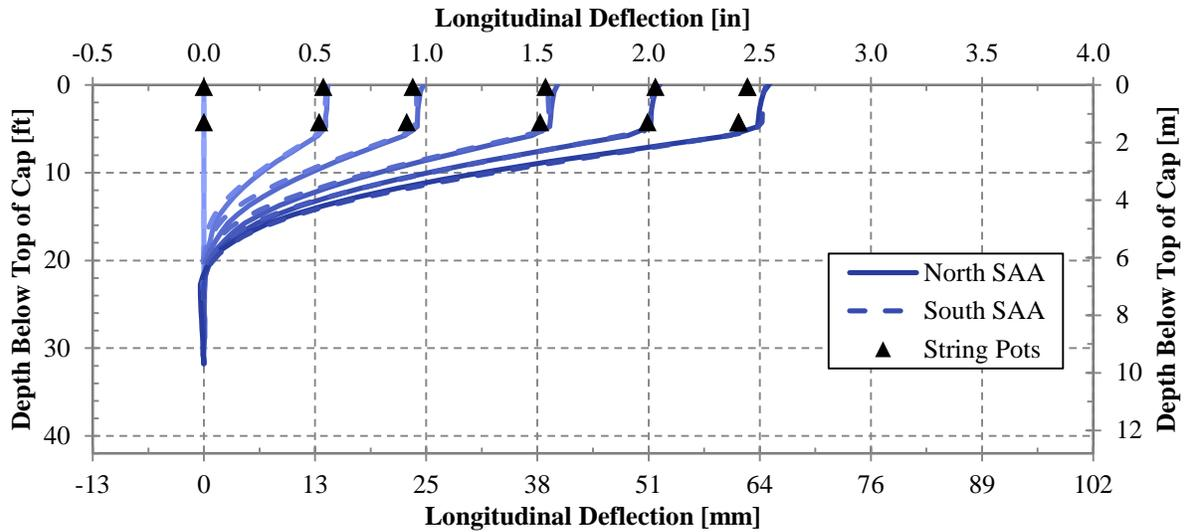
**Figure 20. Longitudinal deflection vs. depth curves for 30° skew 5.5 ft test from string potentiometer and SAA data at various deflection increments**
