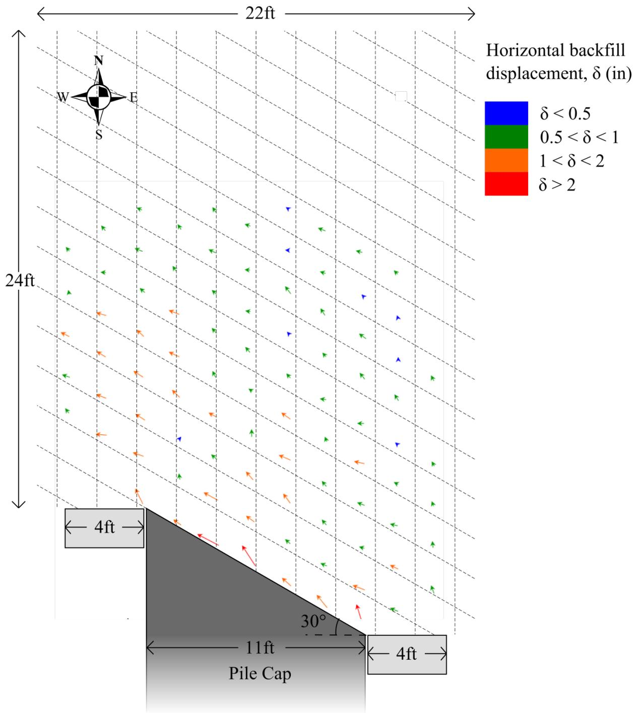
Figure 26. Soil displacement for 30° skew 5.5 ft. gravel backfill unconfined.
