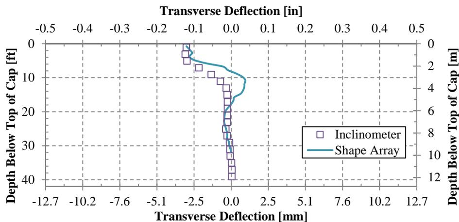
**Figure 17. North 3.5-ft backfill 0° skew final deflections comparing inclinometer and shape array**
