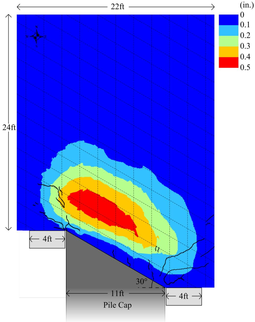
**Figure 24. Heave contours (units in inches) and surface cracks at 2.5 in (7.61 cm) of longitudinal displacement (test completion) for 30° skew (NOTE 1 inch = 2.54 centimeters).**
