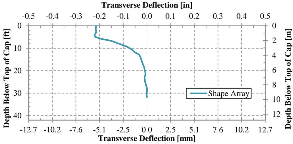
Figure 18. North 5.5-ft backfill 30° skew final deflections according to shape array measurements
