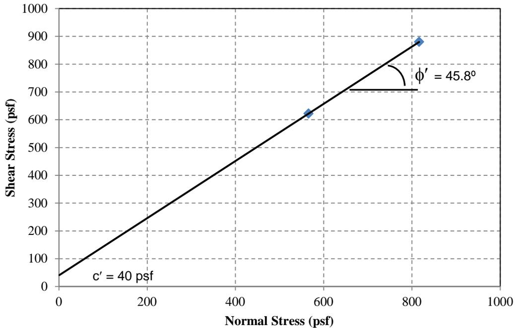
**Figure 11. In situ box direct shear results for gravel backfill**
