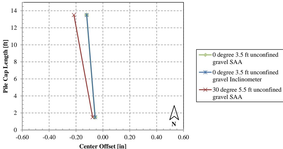
**Figure 21. Transverse pile cap deflection and rotation determined between north and south shape array and inclinometer data**
