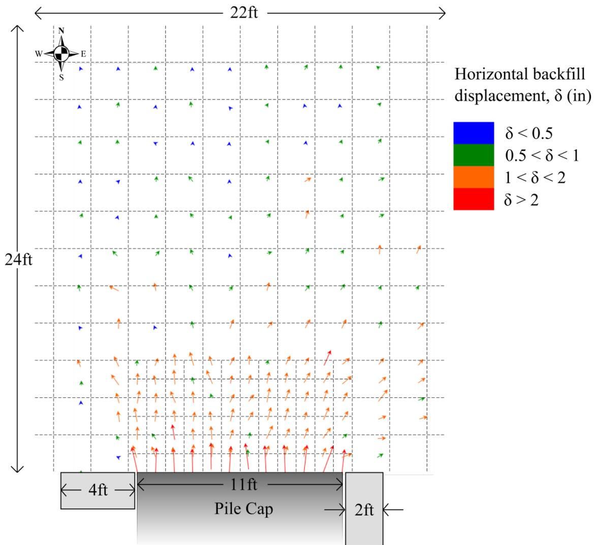
**Figure 25. Soil displacement for 0° skew 3.5 ft. gravel backfill unconfined.**
