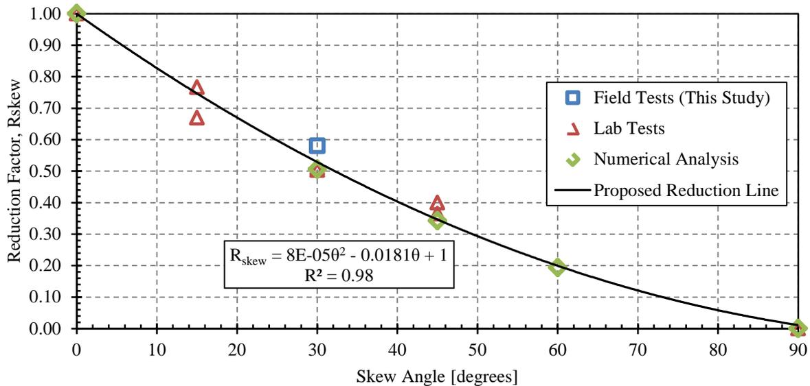
**Figure 14. Reduction factor,  $R_{skew}$  (passive force for a given skew angle normalized by passive force with no skew) plotted versus skew angle based on lab tests (Rollins and Jessee 2012), numerical analyses (Shamsabadi et al. 2006) and results from field tests in this study.**
