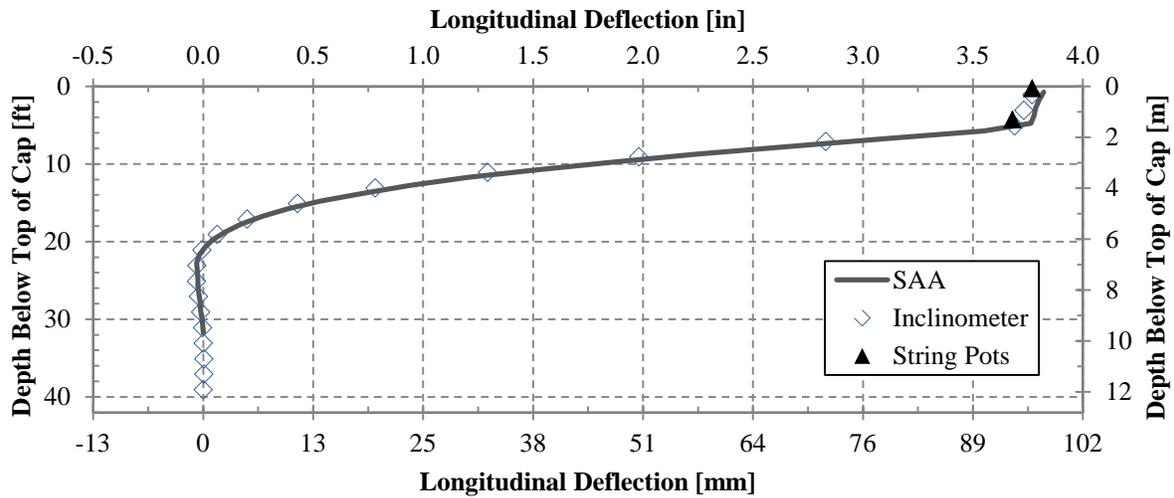
Figure 15. North 3.5-ft backfill 0° skew final deflection comparing inclinometer, shape array, and string potentiometers.
