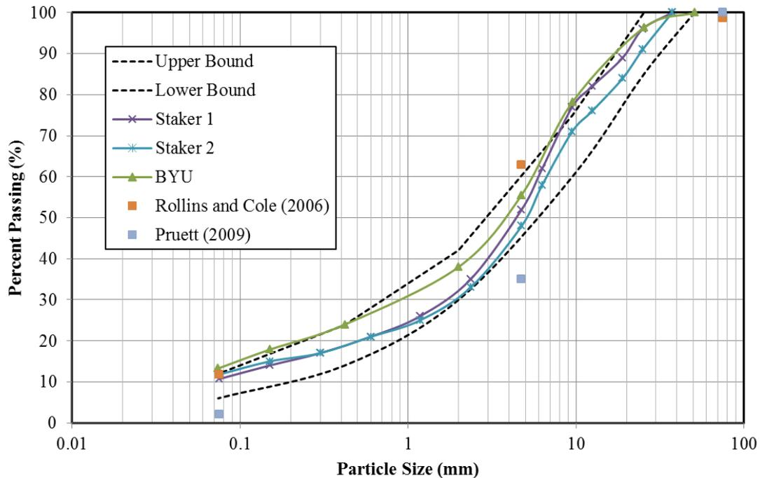
**Figure 5. Gradation for backfill gravel relative to specified limits.**
