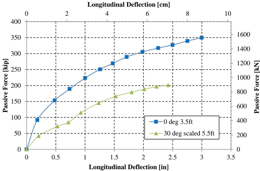
**Figure 13. Comparison of passive force versus longitudinal deflection for 0° and 30° skew**
