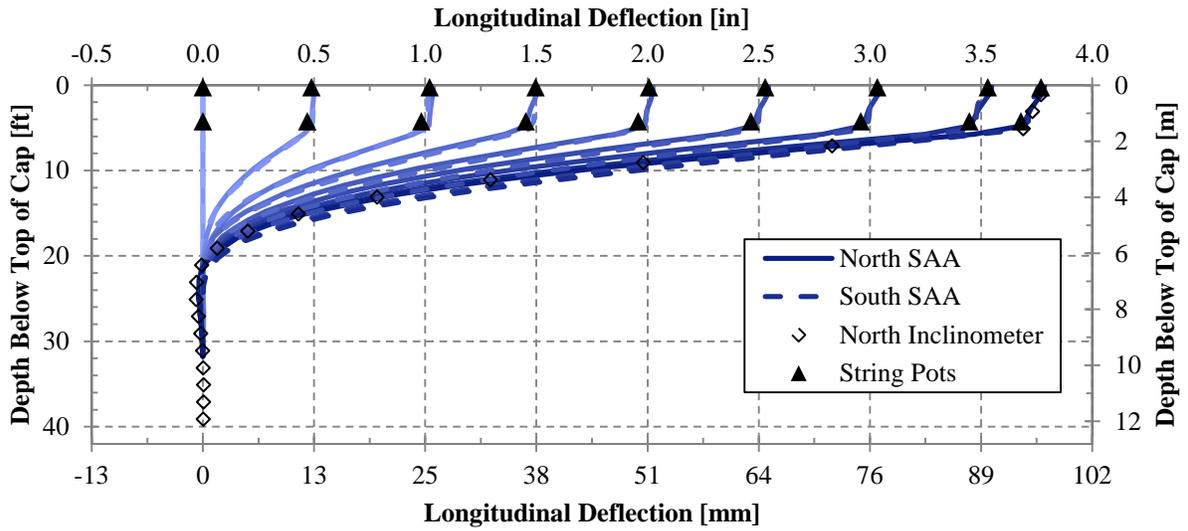
Figure 19. Longitudinal deflection vs. depth curves for 0° skew 3.5 ft test from string potentiometer and SAA data at various deflection increments and the final north inclinometer reading
