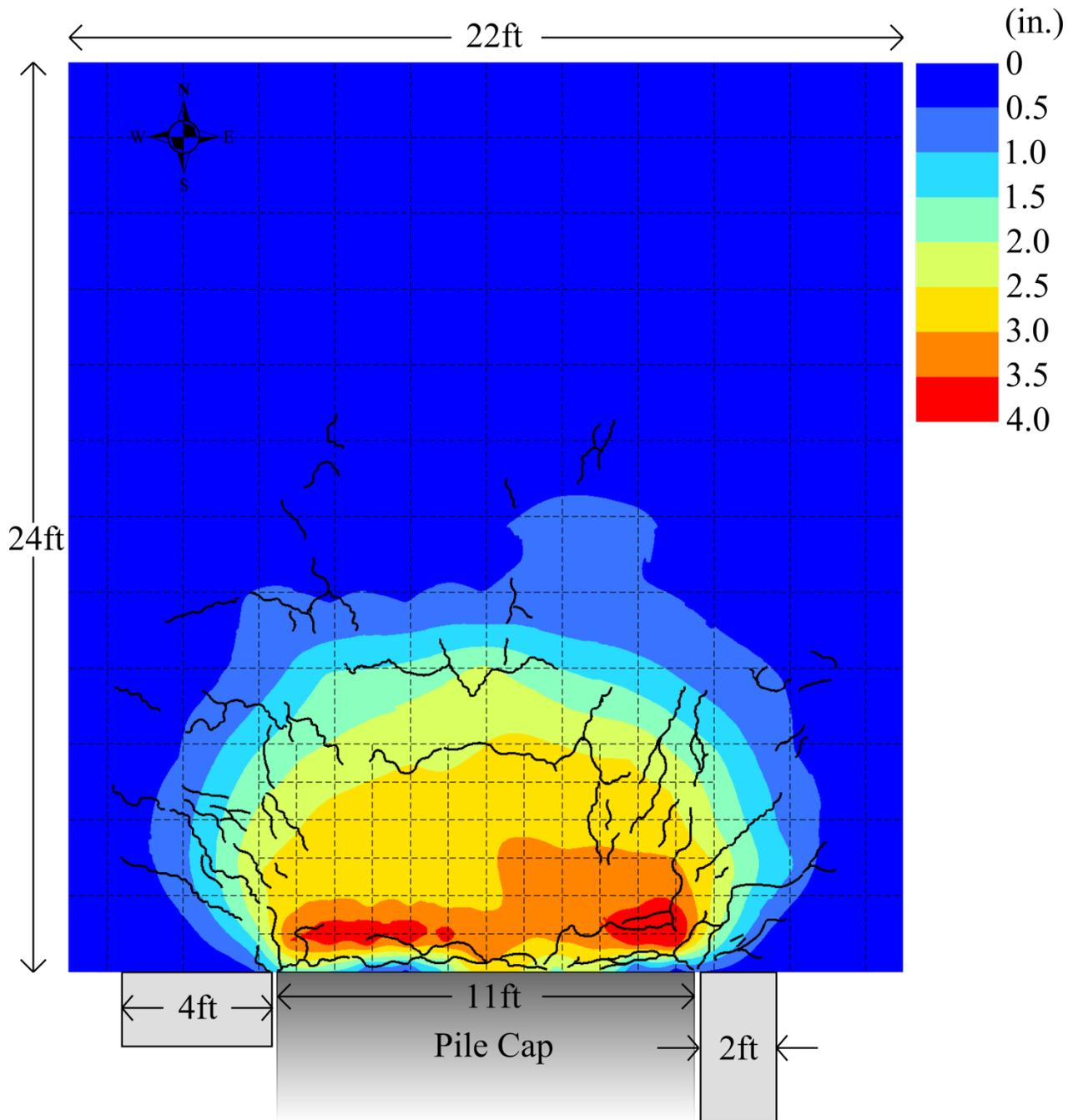
**Figure 23. Heave contours (units in inches) and surface cracks at 3.0 in (7.61 cm) of longitudinal displacement (test completion) for 0° skew test (NOTE: 1 inch = 2.54 centimeters).**
