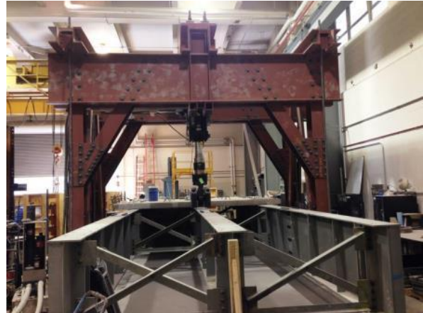
(d) Reaction frame and three-girder test bridge with deck partially removed
