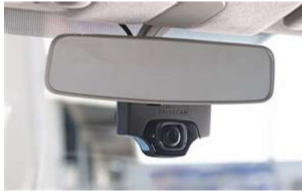
Figure 2. DriveCam Event-Triggered Video Data Recorder
