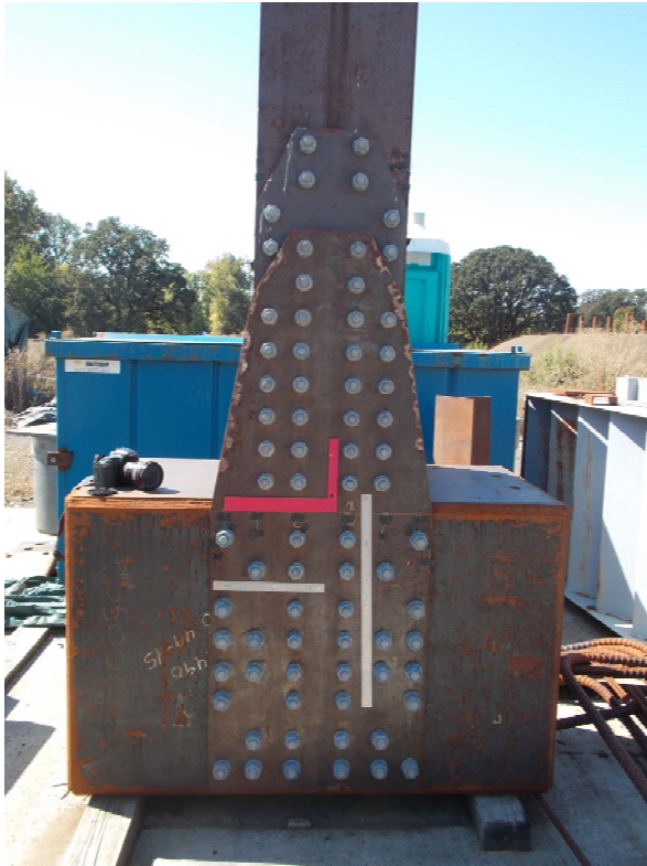
Figure 1. New image target applied to laboratory gusset plate. Straight rules are to verify scale in post-processed images.
