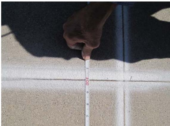
a. Aligning the 20-ft. mark of the guidance tape with the start line
