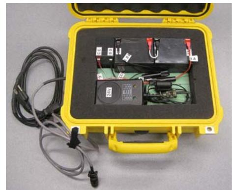
b. Open showing batteries and chargers
