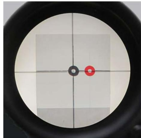
Figure 3.10. View through the sighting scope with the visual field centered and the crosshairs centered within the black circle
