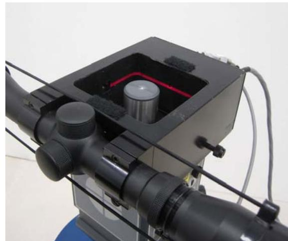
b. Rear quarter view showing the laser beam sweeping across the window into the circuit chamber
