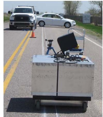
Figure 4.6 Vehicles positioned to block headlights of approaching vehicles
