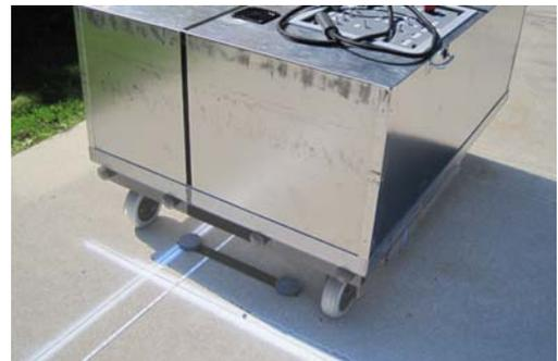
Figure 4.9. The profiler in position to start the measurement of a segment
