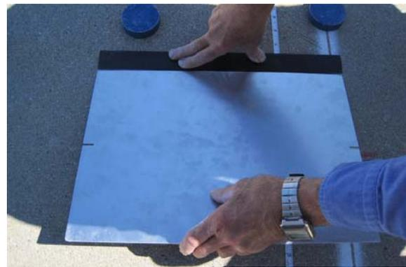
b. Place the transfer plate edge firmly against the marker plate edge
