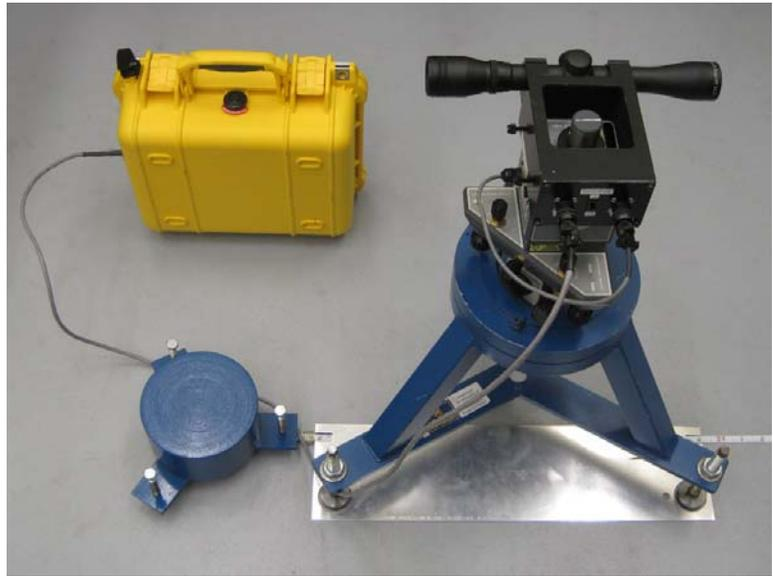
Figure 3.1. The spinning laser assembly, with battery pack, positioned over the guidance tape with the tripod alignment plate
