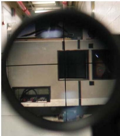
b. View in the sighting scope with the laser leveled and aligned
