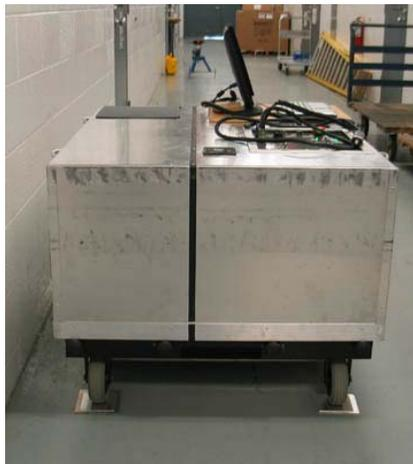
a. Profiler on leveling shims 30 ft. in front of the laser
