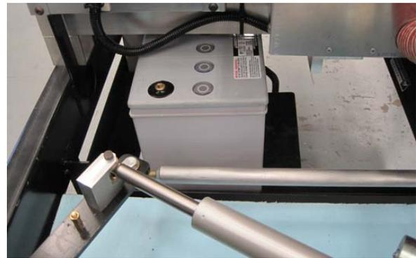
**b. Slide the battery onto the support plate.**
