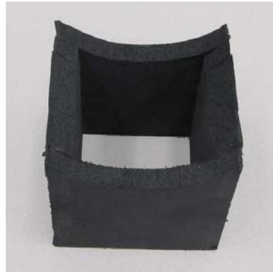
Figure A.15. Sun shade for laser bubble-levels
