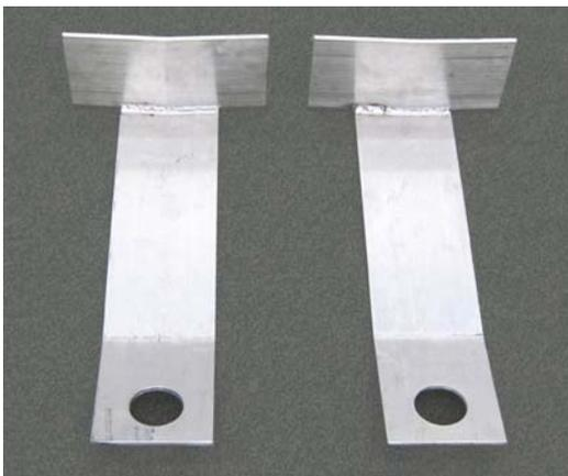
Figure A.16. Stretched-rope anchor plates
