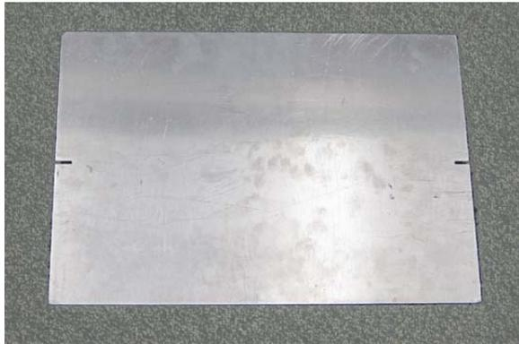
Figure A.14. Marker-strip transfer plate
