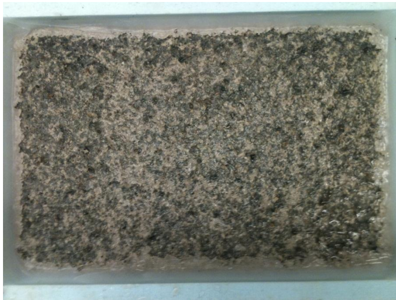
Figure 4. BNQ (VDOT curing) exposure for Mix #13 50%LA 50%SG120 0.42w/c at 25 cycles where finer sized pieces of scale were observed
