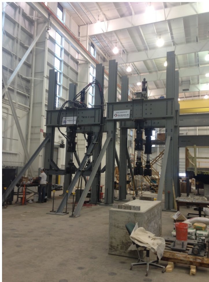
Figure 3: Load Frame setup before completion of hydraulics
