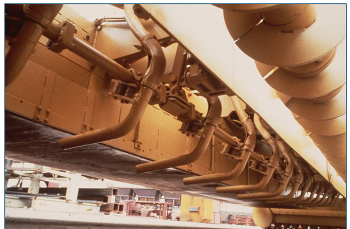
Figure 41. This photo shows a typical line of vibrators mounted to the paver
