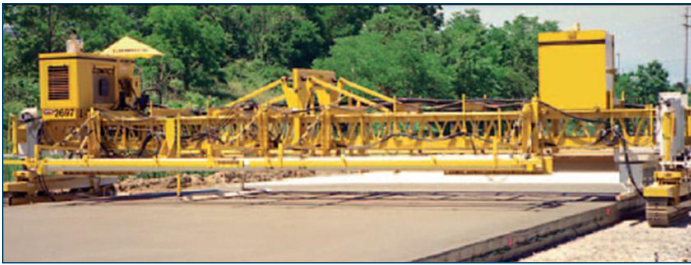
Figure 49. Texture-cure machine manufactured by GOMACO
