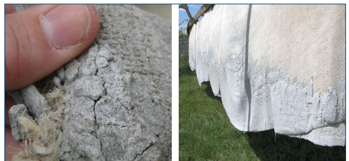
Figure 29. Hardened mortar on drag materials
