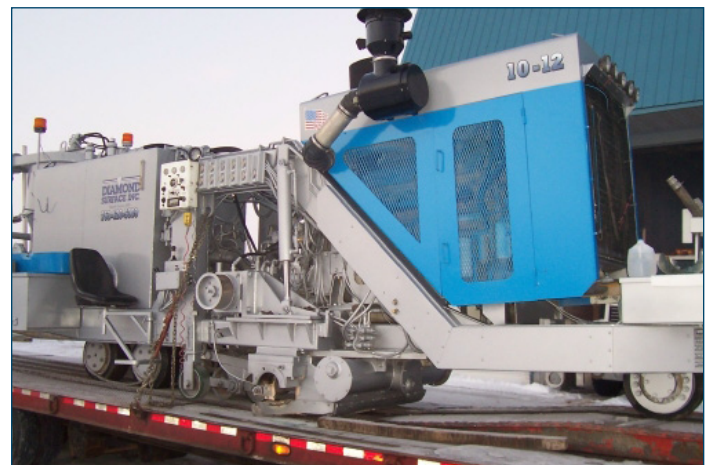
Figure 60. Grinder used for large-scale concrete pavement texturing operations
