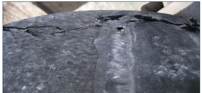
Figure 62. Cracked drive wheel
