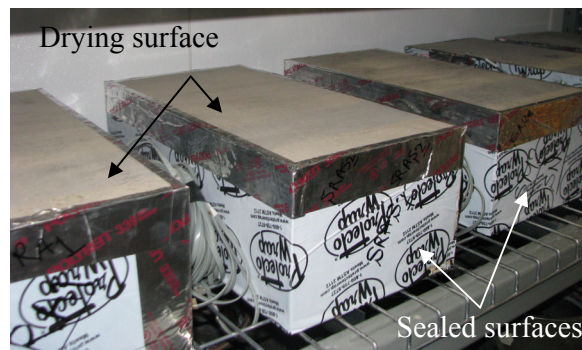
Figure 2: Slab geometry with one-sided drying
