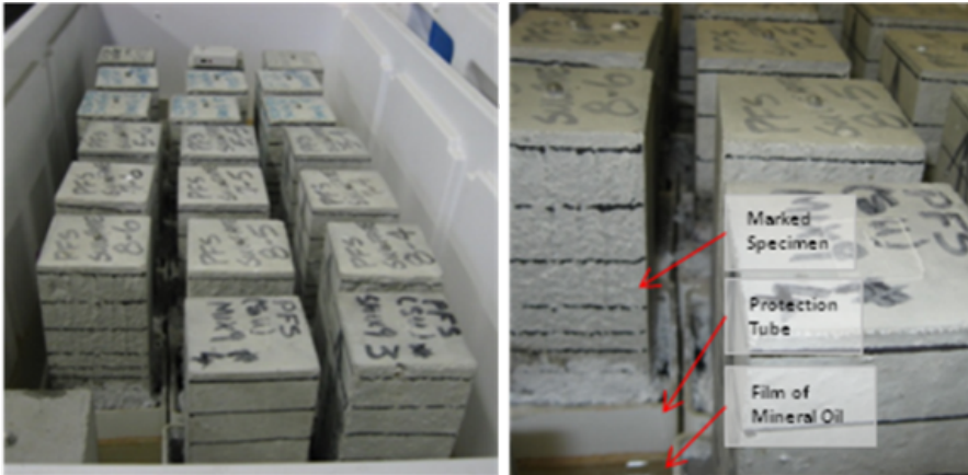
Figure 14 USBR half immersed specimens in the container
