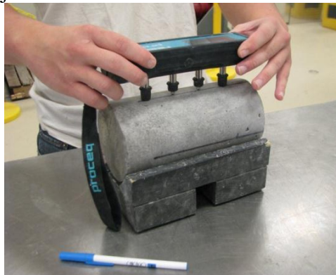
34 Figure 1 – Surface resistivity measurements using a Wenner probe.
