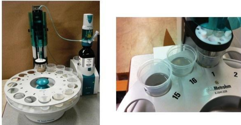
17 18 Figure 7 – Automated titration unit.
