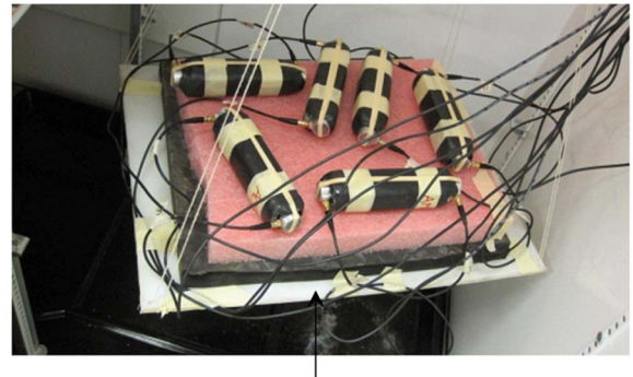
Suspended plate to eliminate vibration and noise from environment
