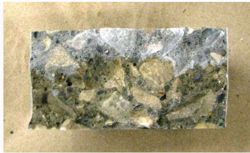
Figure 4 – A Sample from the Rapid Chloride Migration (RCM) test that was split after and sprayed with Silver Nitrate (AgNO 3 ). The white portion of the sample at the top represents the chloride penetration while the brown area represents the portion of the concrete that has not received substantial chloride penetration. The sample is 101 mm (4 in wide) and 50 mm (2 in tall).
