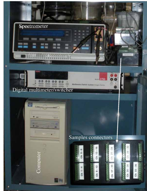
Fig. 2. Components of the system.
