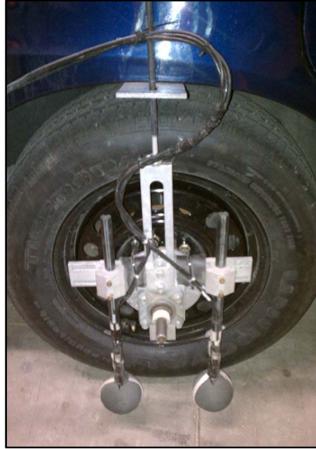
Figure 1. On-Board Sound Intensity Test Setup.
