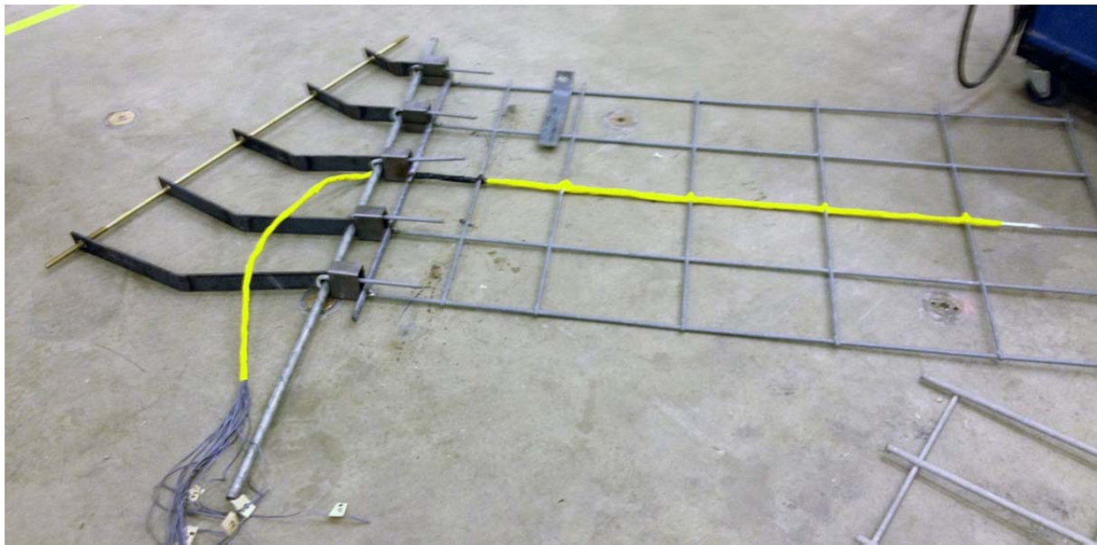
Figure 3.19: Angled Adapter Connectors attached to Reinforcement Grids to Accommodate the Skewed Shape
