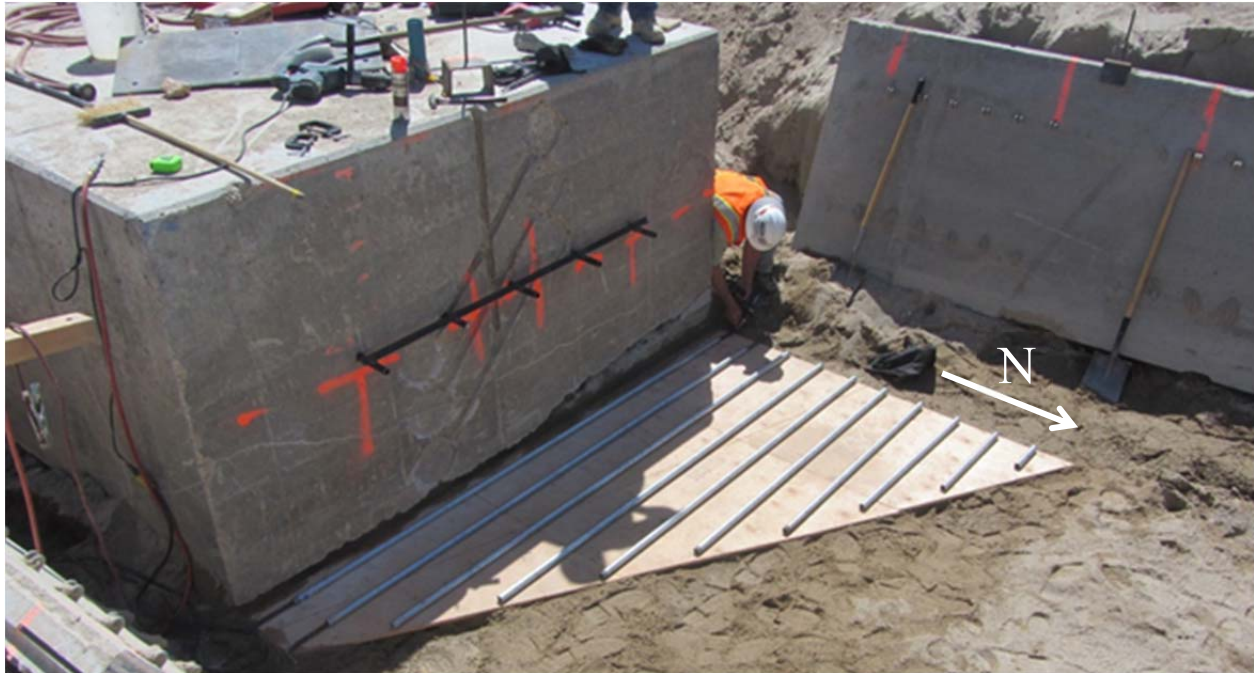
Figure 3.11: Steel Roller Bearing Platform for Concrete Wedges
