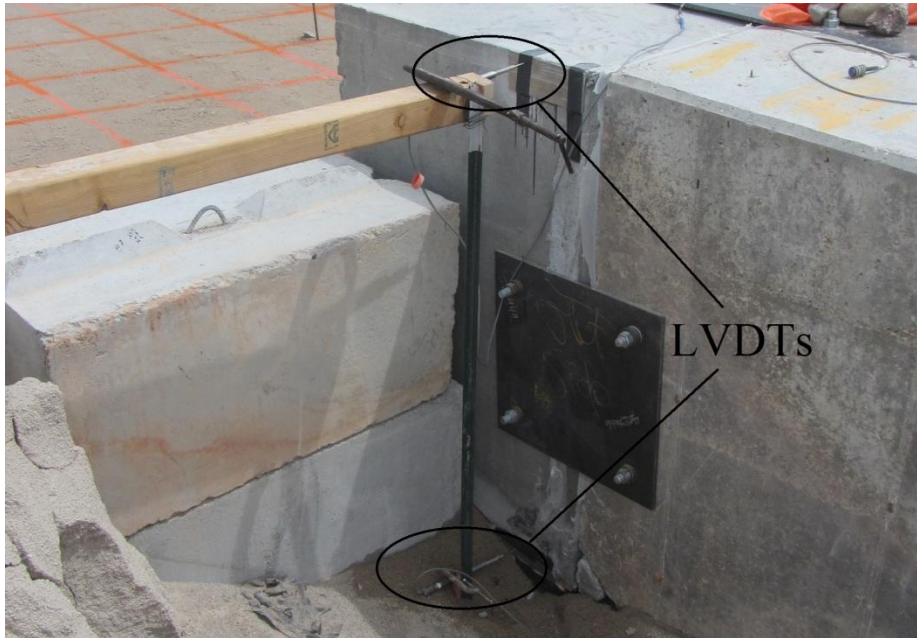
Figure 3-15: LVDTs for measuring transverse cap movement (north end)
