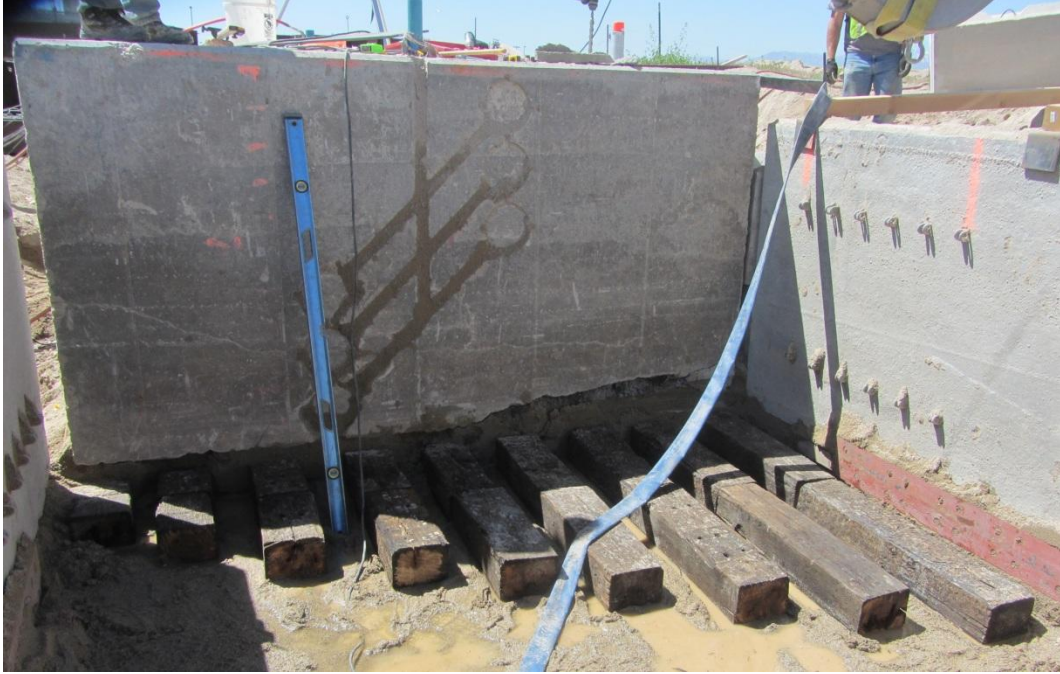
Figure 3-9: Railroad tie foundation for 15° and 30° wedges
