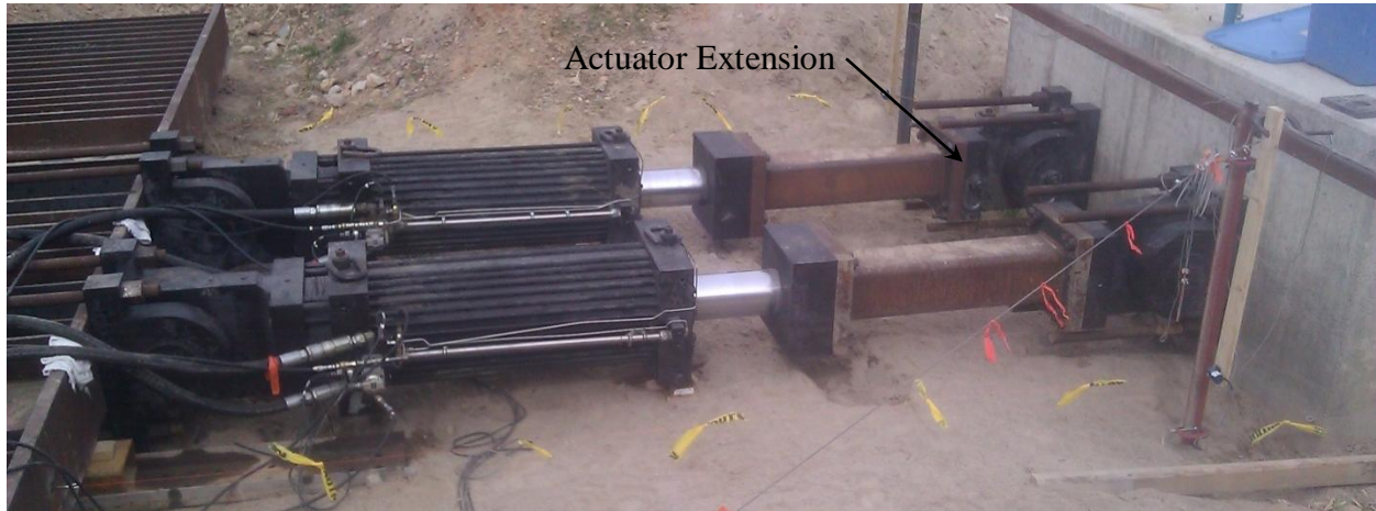
Figure 3-13: MTS hydraulic actuators
