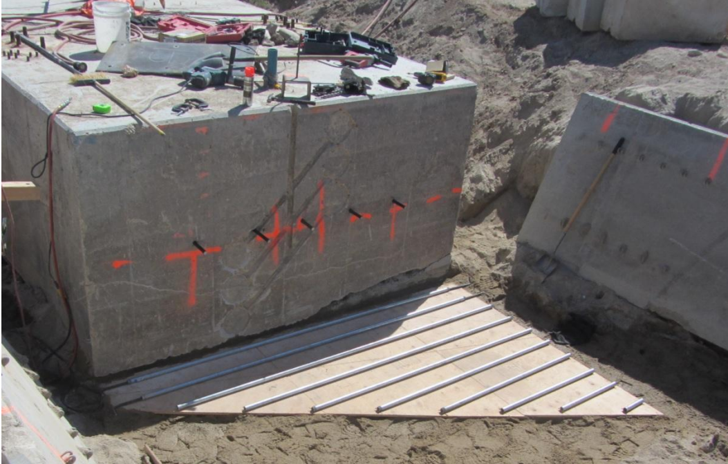
Figure 3-11: Roller foundation for 15° and 30° wedges
