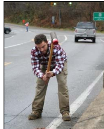
Figure 2-10 – Manual Impact at Smithers Bridge
