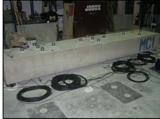
Figure D 2 - Concrete Beam Test
