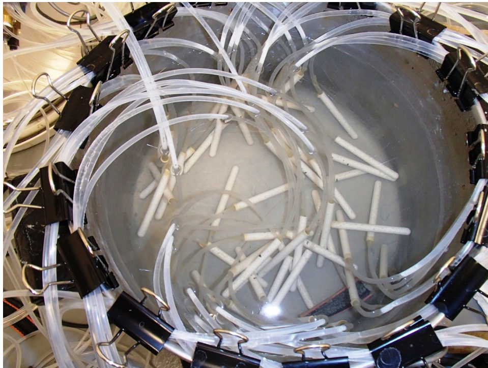
Figure 37: Saturation of ceramic porous stones.
