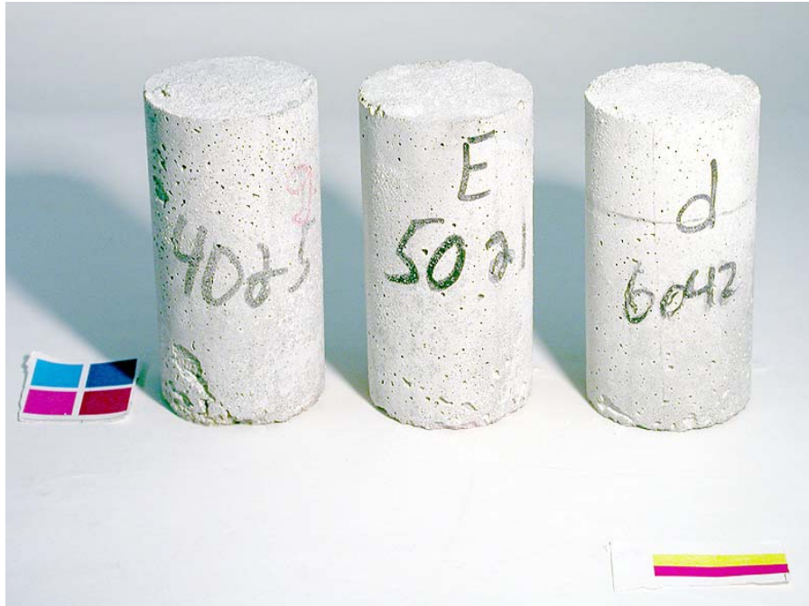
Figure 3.71. Cylinders exposed to CMA solution after 84 days of constant low temperature test. From left to right: 0.40, 0.50, and 0.60 w/c mortar cylinders.
