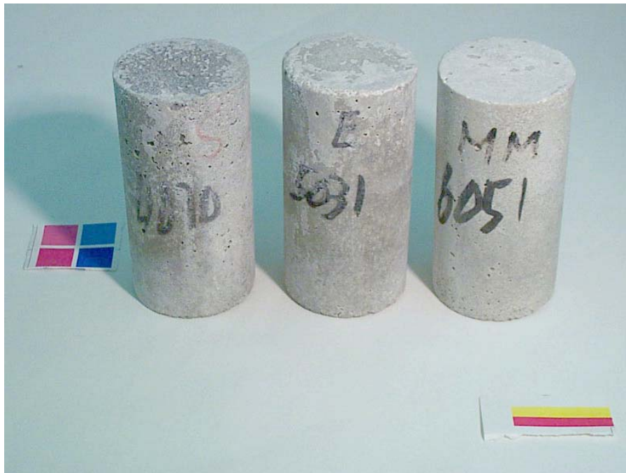
Figure 3.111. Cylinders exposed to CaCl_2 solution after 84 days of constant high temperature test. From left to right: 0.40, 0.50, and 0.60 w/c mortar cylinders.
