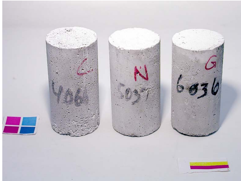
Figure 3.125. Cylinders exposed to \text{CaCl}_2 solution after 56 days of constant low temperature test. From left to right: 0.40, 0.50, and 0.60 w/c mortar cylinders. Solution strength was 3% \text{CaCl}_2 .
