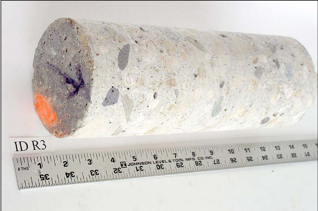
Figure 3.4. Core as received from Idaho site, left-most lane, at joint, (ID_R03).
