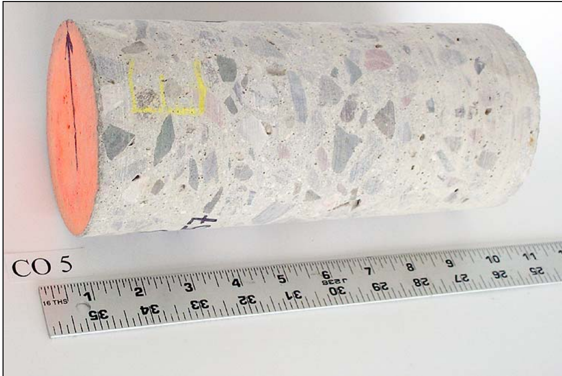
Figure 3.20. Core as received from Colorado site, away from joint (CO_05).
