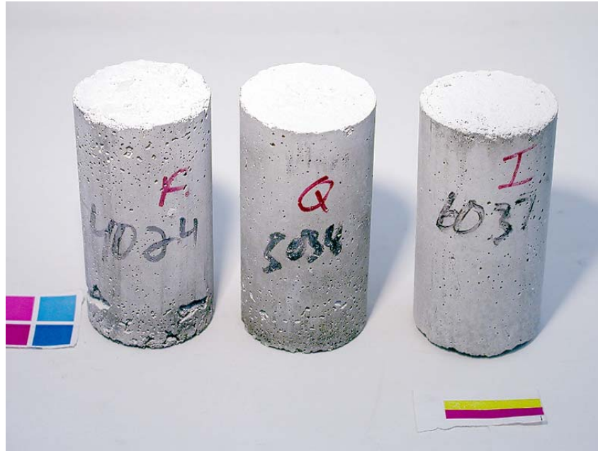
Figure 3.127. Cylinders exposed to \text{CaCl}_2 solution after 56 days of constant low temperature test. From left to right: 0.40, 0.50, and 0.60 w/c mortar cylinders. Solution strength was 10% \text{CaCl}_2 .
