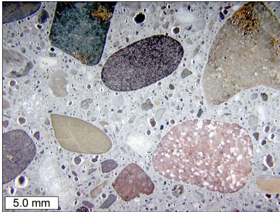
Figure 3.17. Stereomicroscope image of polished surface from core MT_02, magnified here approximately 4x.
