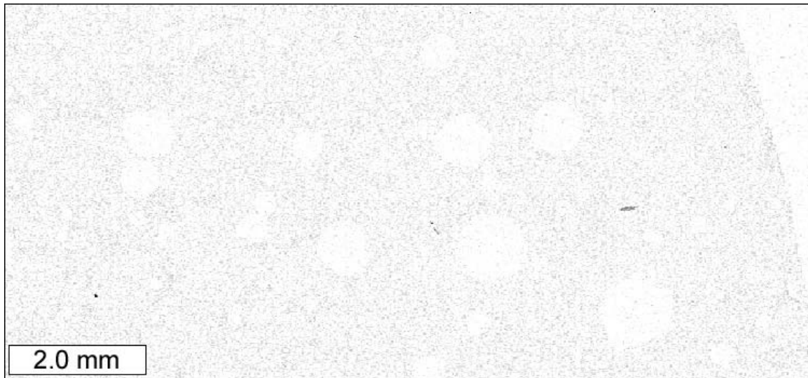
Figure 3.61a: Potassium K\alpha x-ray map from control cylinder. Darker areas correspond to higher K\alpha x-ray counts.
