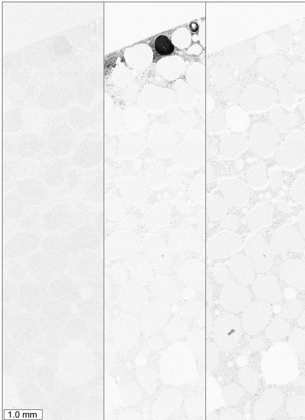
Figure 3.86: Elemental maps, from left to right: sodium, magnesium, and aluminum. The elemental maps were collected from a thin section prepared from a cylinder immersed in magnesium chloride solution.
