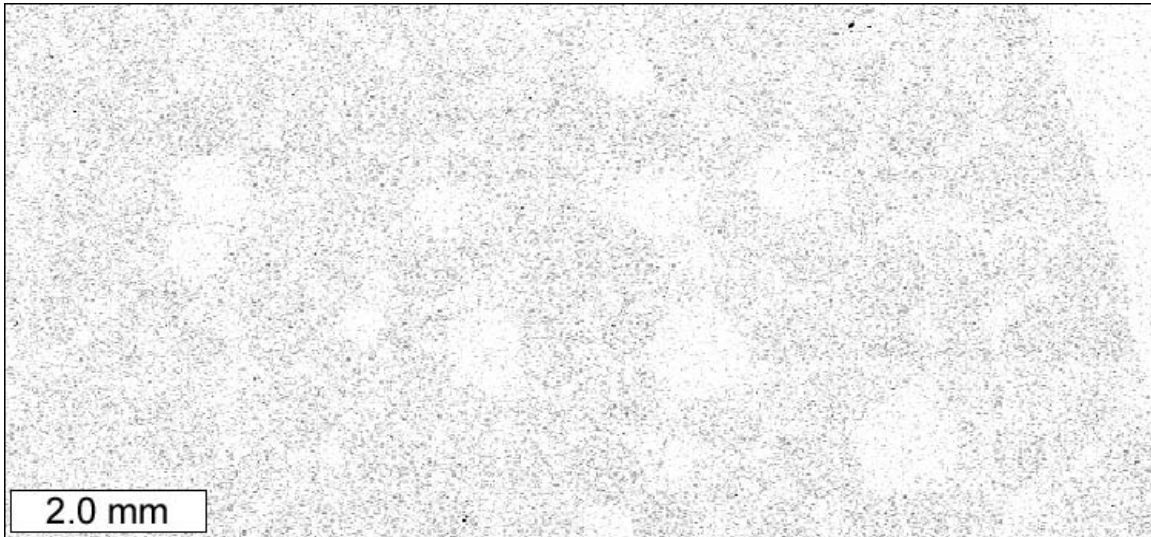
Figure 3.55a: Sodium K\alpha x-ray map from control cylinder. Darker areas correspond to higher K\alpha x-ray counts.
