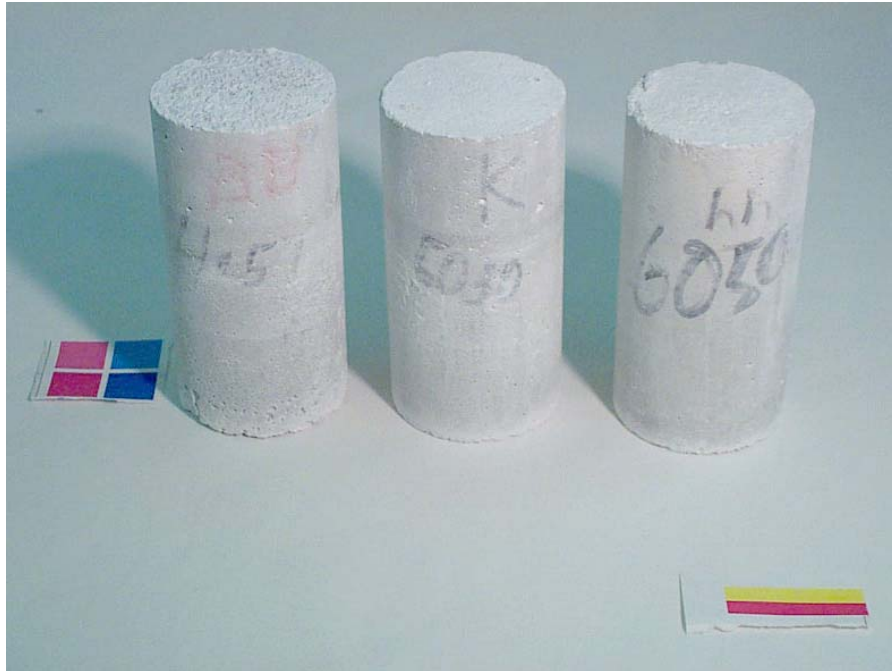
Figure 3.49. Control cylinders exposed to lime water solution after 84 days of cyclic temperature test. From left to right 0.40, 0.50, and 0.60 w/c mortar cylinders.
