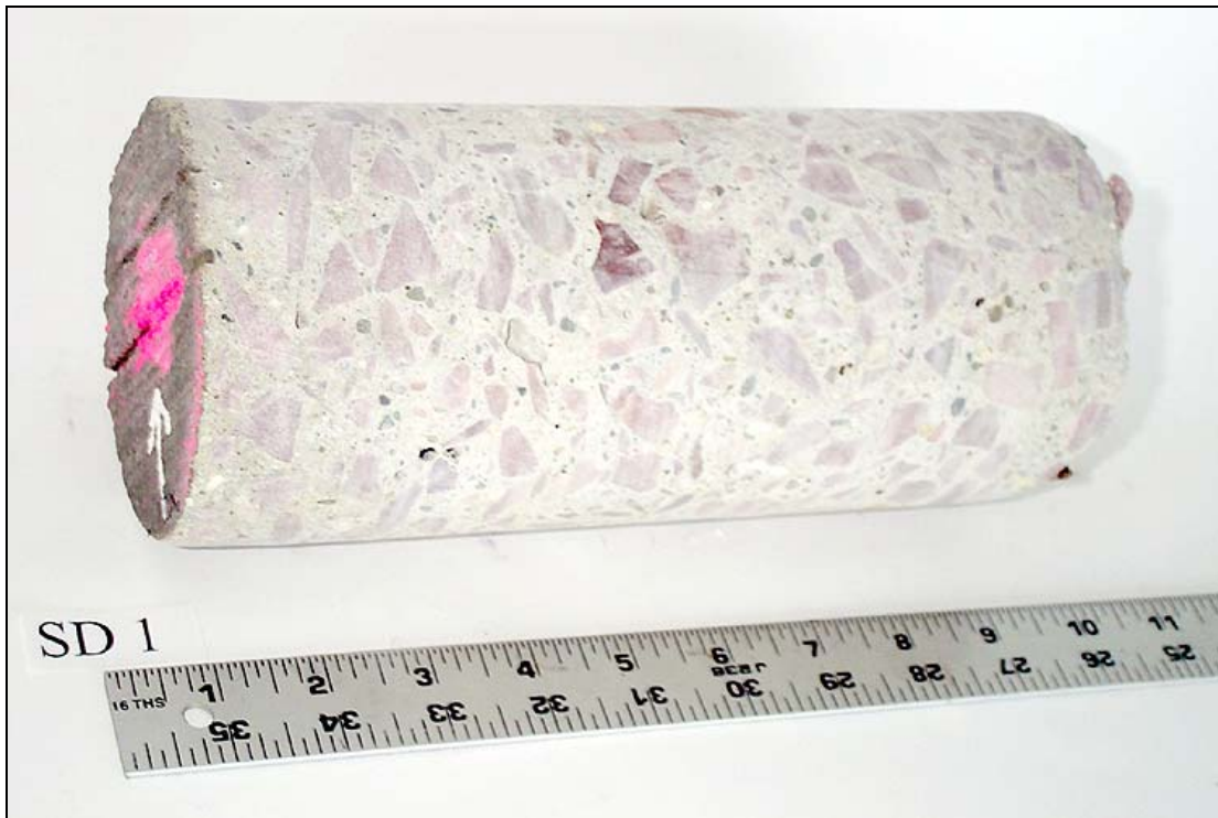
Figure 3.26. Core as received from South Dakota site, at joint (SD_01).
