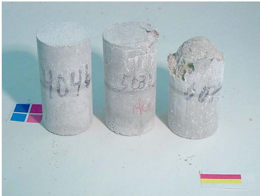
Figure 3.44 Cylinders exposed to MgCl_2 solution after 56 days of cyclic temperature test. From left to right: 0.40, 0.50, and 0.60 w/c mortar cylinders
