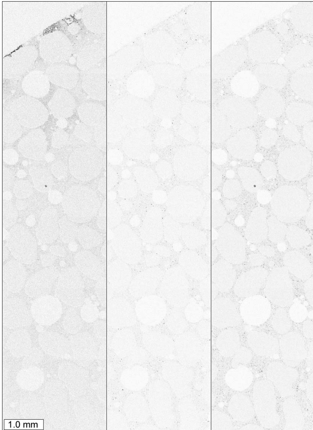
Figure 3.96: Elemental maps, from left to right: sodium, magnesium, and aluminum. The elemental maps were collected from a thin section prepared from a cylinder immersed in sodium chloride solution.
