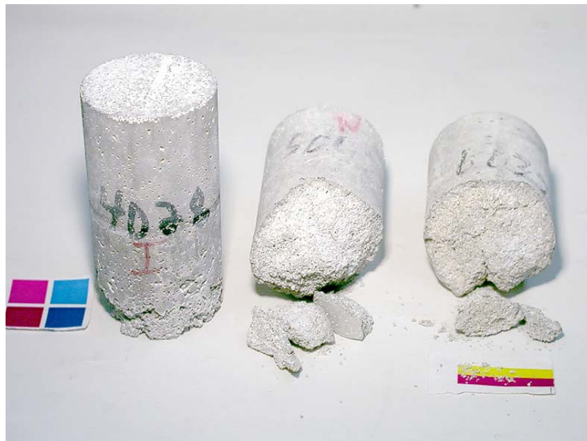
Figure 3.123. Cylinders exposed to rock salt NaCl solution after 56 days of cyclic temperature test without the oven step. From left to right: 0.40, 0.50, and 0.60 w/c mortar cylinders.
