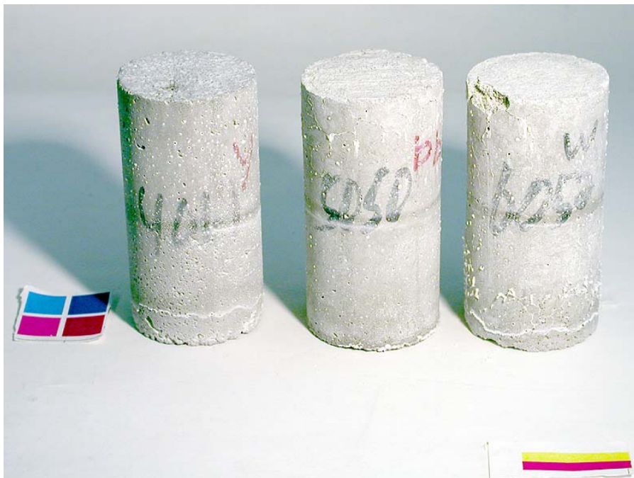
Figure 3.48. Cylinders exposed to CMA solution after 84 days of cyclic temperature test. From left to right: 0.40, 0.50, and 0.60 w/c mortar cylinders.
