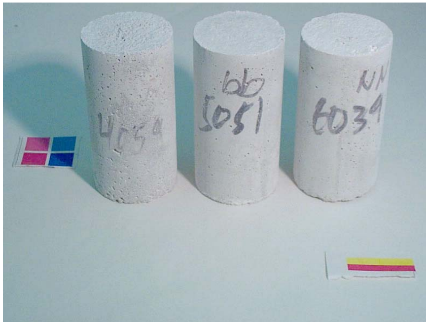
Figure 3.113. Control cylinders exposed to lime solution after 84 days of constant high temperature test. From left to right: 0.40, 0.50, and 0.60 w/c mortar cylinders.
