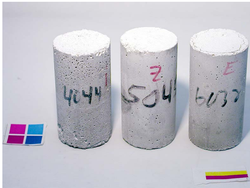
Figure 3.126. Cylinders exposed to \text{CaCl}_2 solution after 56 days of constant low temperature test. From left to right: 0.40, 0.50, and 0.60 w/c mortar cylinders. Solution strength was 7% \text{CaCl}_2 .
