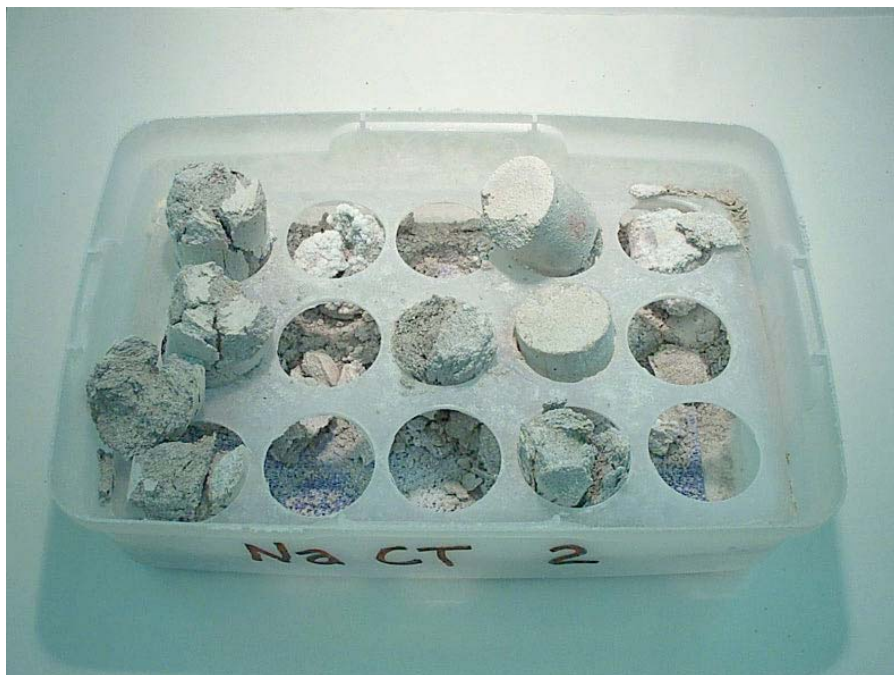
Figure 3.42 Cylinders exposed to rock salt NaCl solution in drained tray after 28 days of cyclic temperature test.
