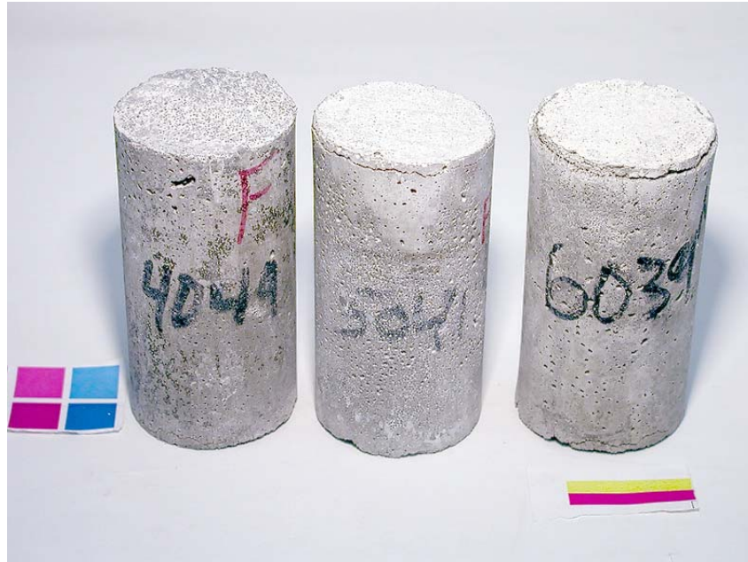
Figure 3.124. Cylinders exposed to rock salt NaCl solution after 56 days of cyclic temperature test without the oven step or the conditioning in lime water step. From left to right: 0.40, 0.50, and 0.60 w/c mortar cylinders.
