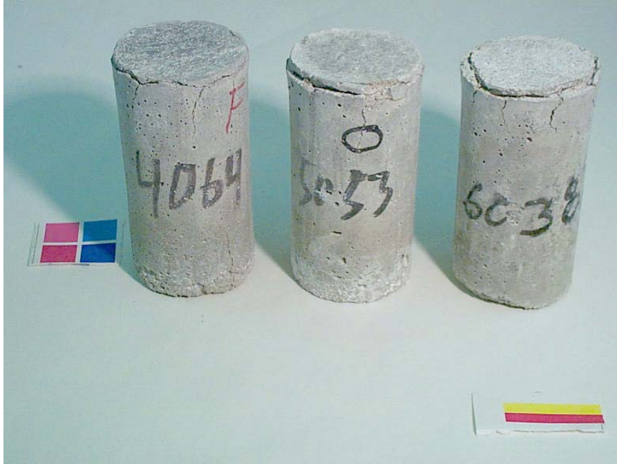
Figure 3.69 Cylinders exposed to MgCl_2 solution after 84 days of constant low temperature test. From left to right: 0.40, 0.50, and 0.60 w/c mortar cylinders.
