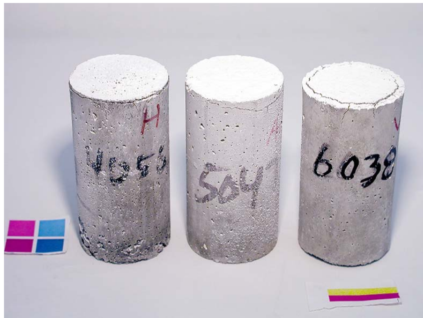
Figure 3.128. Cylinders exposed to \text{CaCl}_2 solution after 56 days of constant low temperature test. From left to right: 0.40, 0.50, and 0.60 w/c mortar cylinders. Solution strength was 14% \text{CaCl}_2 .
