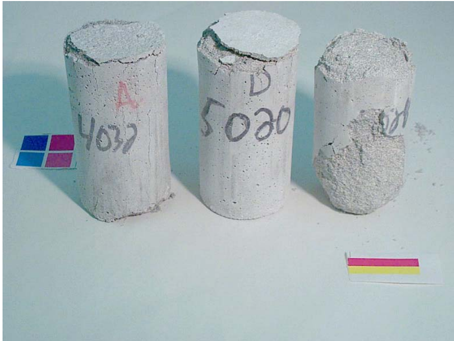
Figure 3.41. Cylinders exposed to food grade NaCl solution after 8 days of cyclic temperature test. From left to right: 0.40, 0.50, and 0.60 w/c mortar cylinders.
