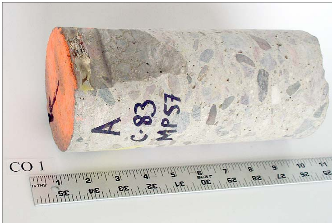
Figure 3.19. Core as received from Colorado site, at joint (CO_01).
