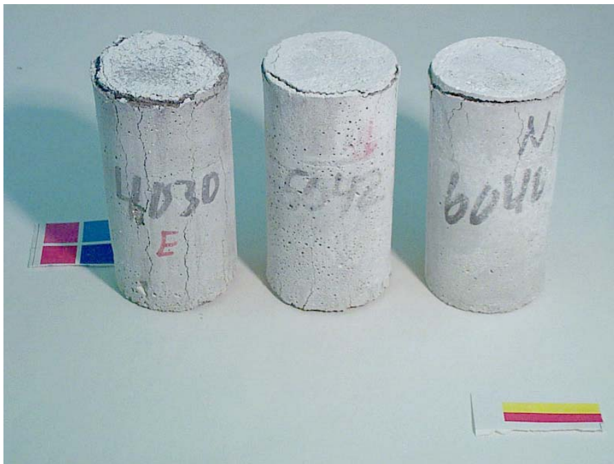
Figure 3.68 Cylinders exposed to CaCl_2 solution after 56 days of constant low temperature test. From left to right: 0.40, 0.50, and 0.60 w/c mortar cylinders.
