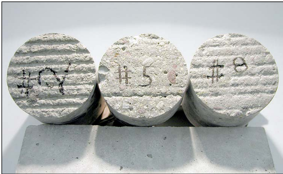
Figure 3.14. Variable wear of pavement surface at Montana site.
