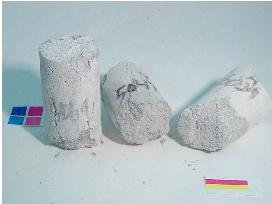
Figure 3.40. Cylinders exposed to rock salt NaCl solution after 8 days of cyclic temperature test. From left to right: 0.40, 0.50, and 0.60 w/c mortar cylinders.
