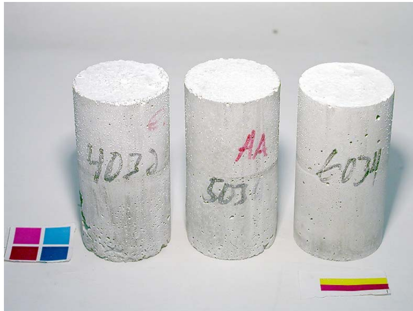
Figure 3.121. Cylinders exposed to rock salt NaCl solution after 28 days of cyclic temperature test without the oven step. From left to right: 0.40, 0.50, and 0.60 w/c mortar cylinders.
