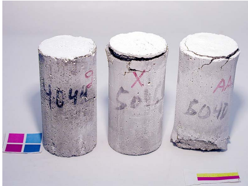
Figure 3.129. Cylinders exposed to \text{CaCl}_2 solution after 56 days of constant low temperature test. From left to right: 0.40, 0.50, and 0.60 w/c mortar cylinders. Solution strength was 17% \text{CaCl}_2 .
