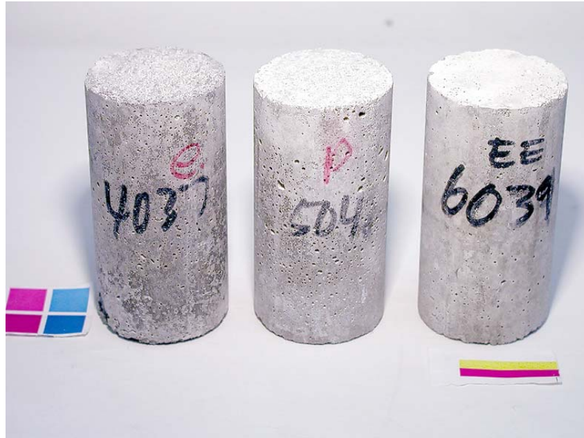
Figure 3.122. Cylinders exposed to rock salt NaCl solution after 28 days of cyclic temperature test without the oven step or the conditioning in lime water step. From left to right: 0.40, 0.50, and 0.60 w/c mortar cylinders.
