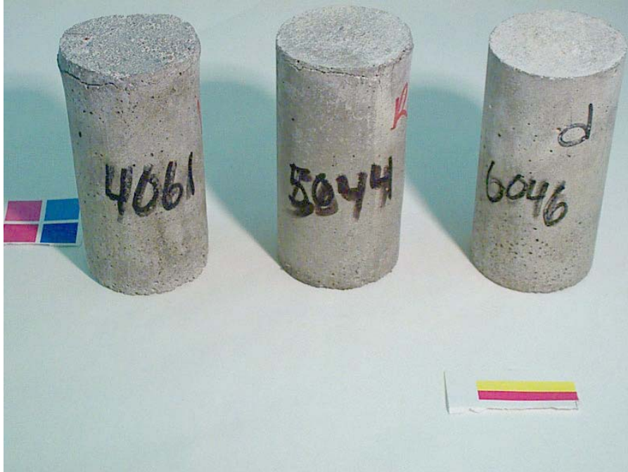
Figure 3.67. Cylinders exposed to MgCl_2 solution after 56 days of constant low temperature test. From left to right: 0.40, 0.50, and 0.60 w/c mortar cylinders.
