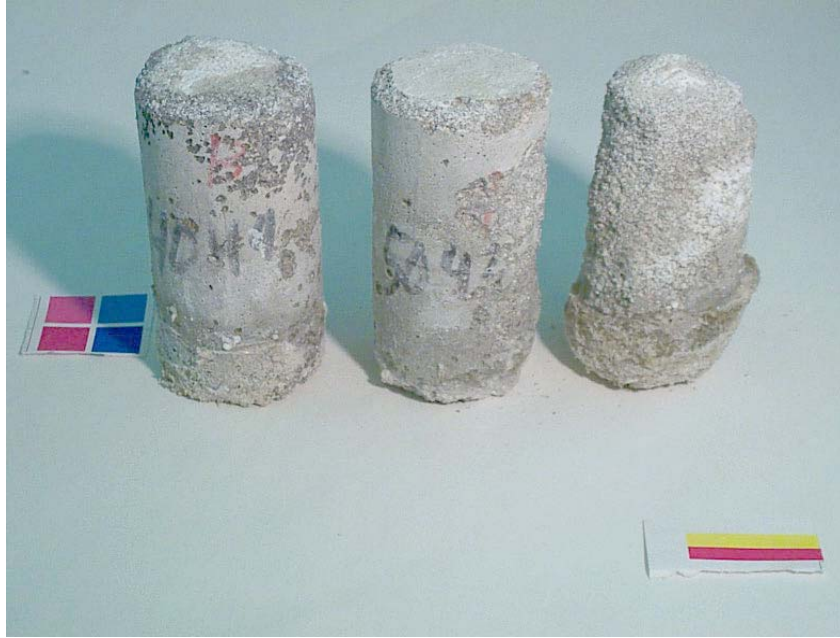
Figure 3.112. Cylinders exposed to CMA solution after 28 days of constant high temperature test. From left to right: 0.40, 0.50, and 0.60 w/c mortar cylinders.
