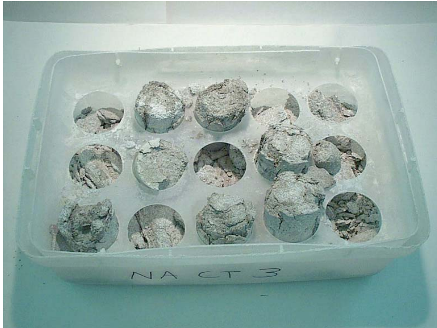
Figure 3.43 Cylinders exposed to food grade NaCl solution in drained tray after 28 days of cyclic temperature test.
