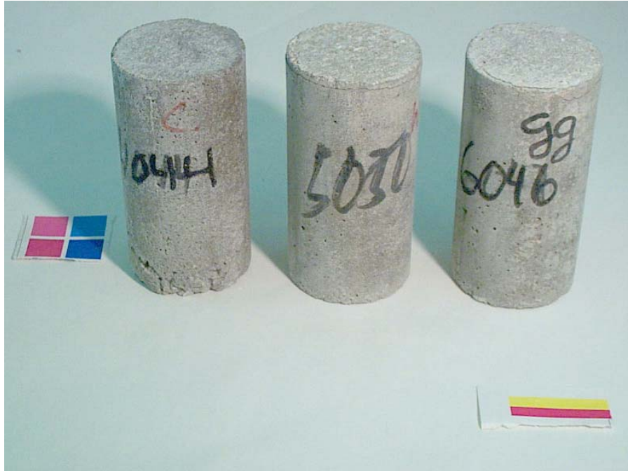
Figure 3.110. Cylinders exposed to MgCl_2 solution after 84 days of constant high temperature test. From left to right: 0.40, 0.50, and 0.60 w/c mortar cylinders.
