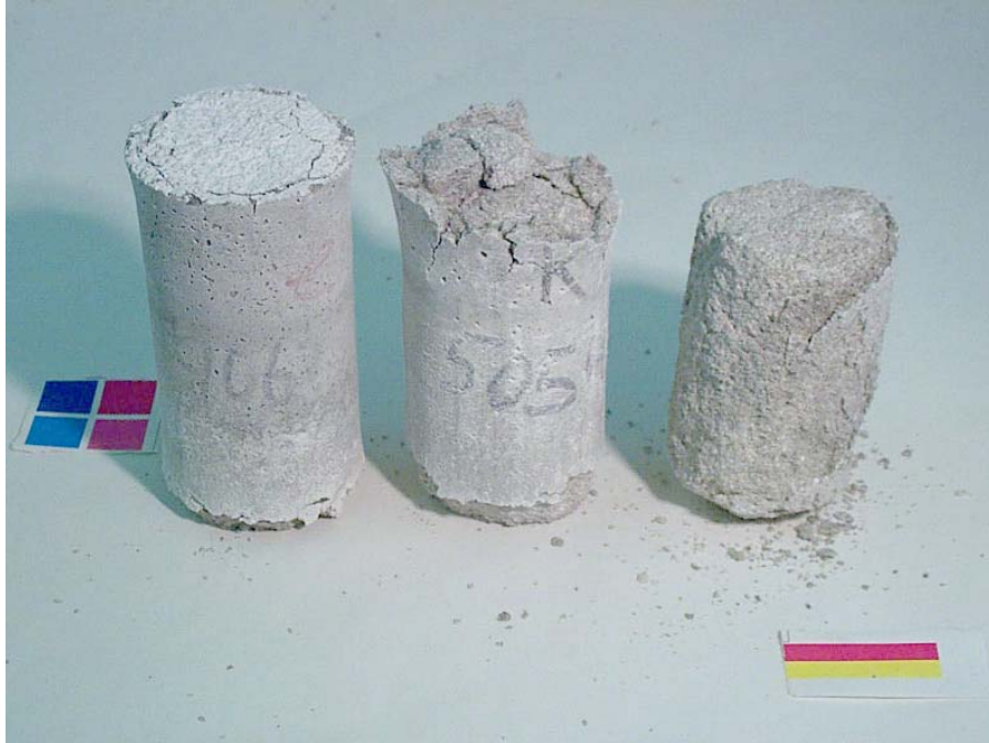
Figure 3.47. Cylinders exposed to \text{CaCl}_2 solution after 84 days of cyclic temperature test. From left to right: 0.40, 0.50, and 0.60 w/c mortar cylinders.
