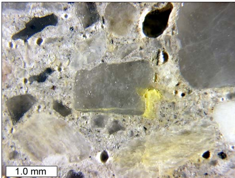
Figure 3.25. Stereomicroscope image of polished surface from core CO_05 showing alkali-silica reactive sand particle after staining procedure.
