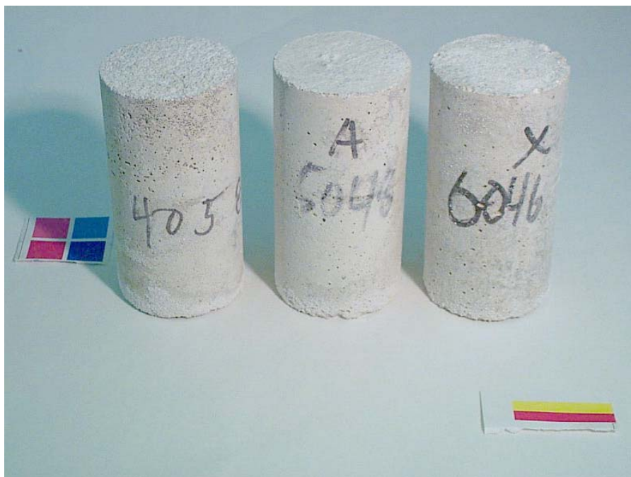
Figure 3.109. Cylinders exposed to NaCl solution after 84 days of constant high temperature test. From left to right: 0.40, 0.50, and 0.60 w/c mortar cylinders.
