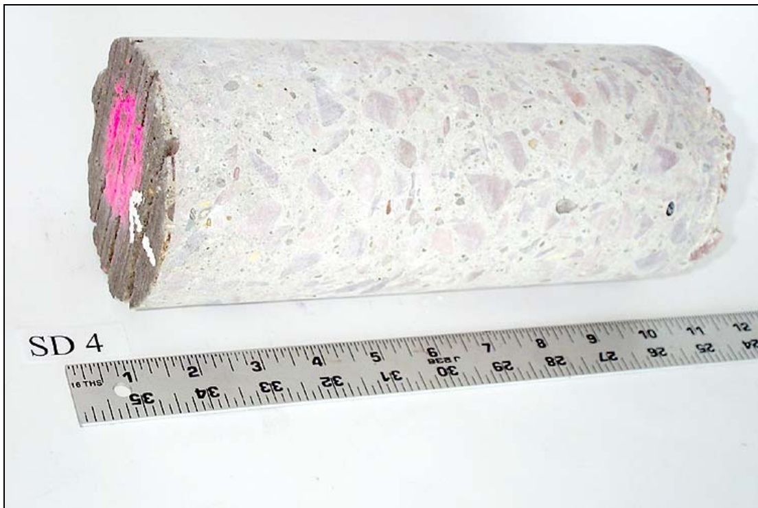
Figure 3.27. Core as received from South Dakota site, away from joint (SD_04).
