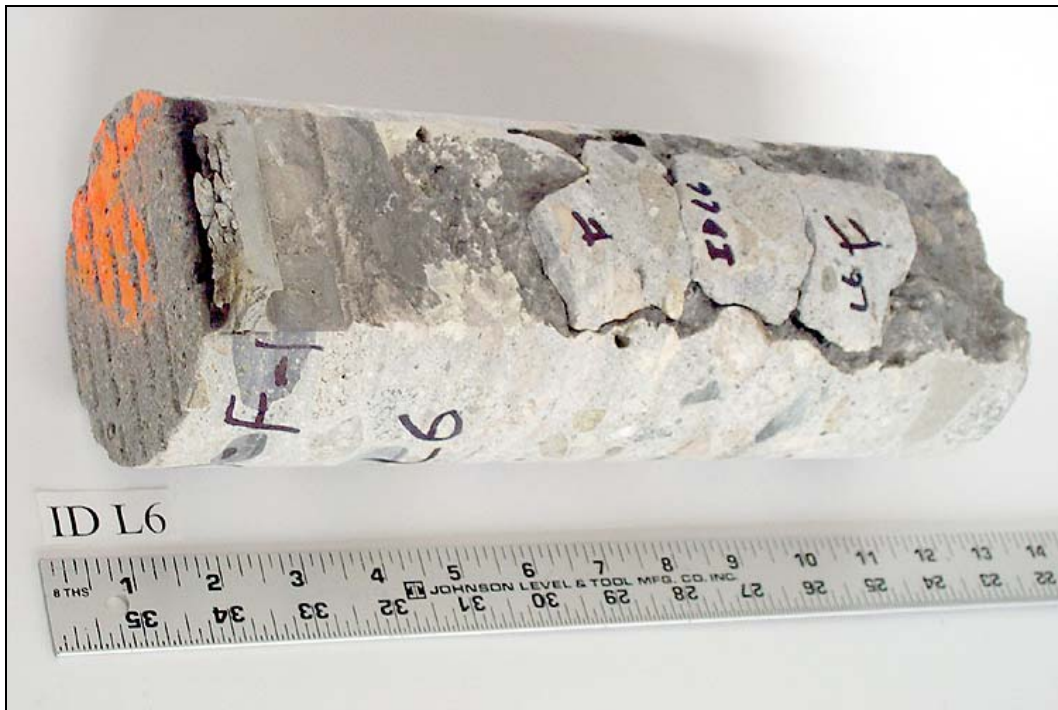
Figure 3.1. Core as received from Idaho site, left-most lane, at joint, (ID_L06).
