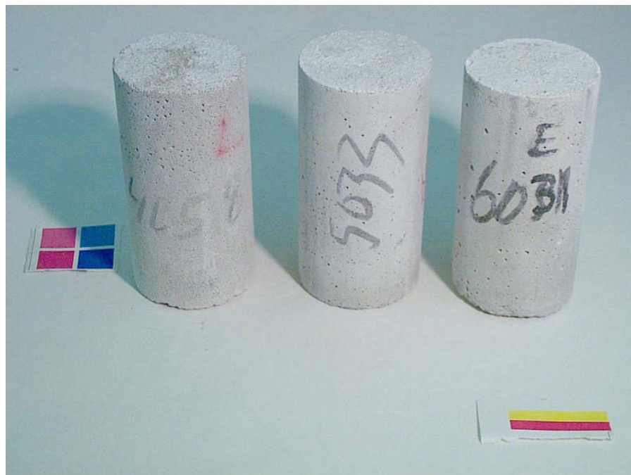
Figure 3.72 Control cylinders exposed to lime water solution after 84 days of constant low temperature test. From left to right: 0.40, 0.50, and 0.60 w/c mortar cylinders.
