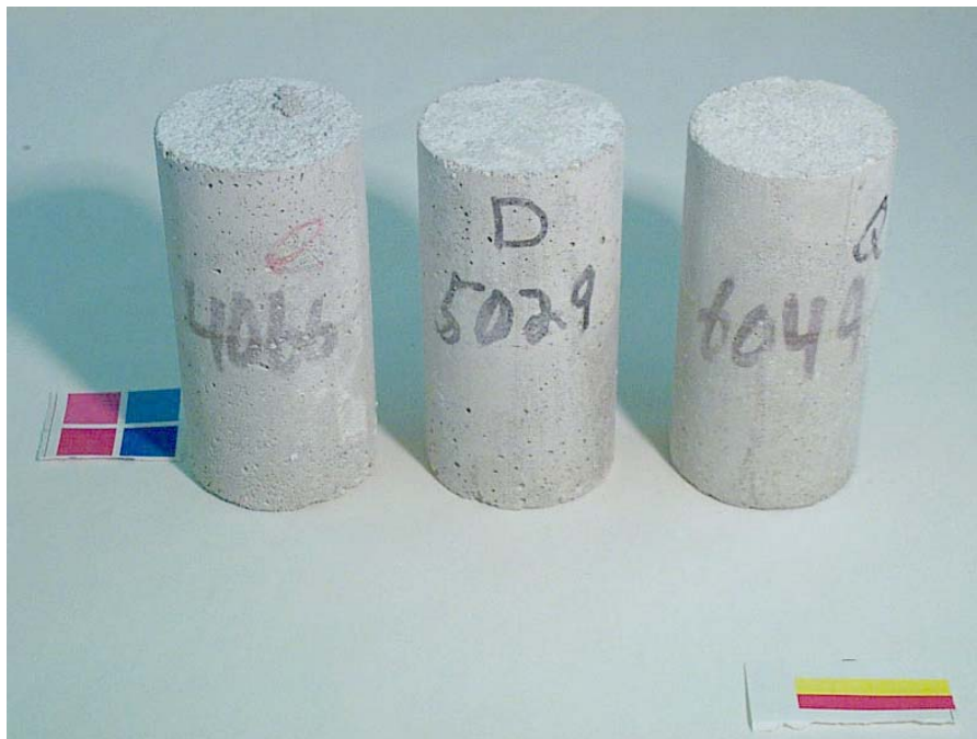
Figure 3.66 Cylinders exposed to NaCl solution after 84 days of constant low temperature test. From left to right: 0.40, 0.50, and 0.60 w/c mortar cylinders.
