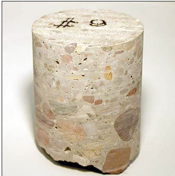
Figure 3.16. Core as received from Montana site, with some surface wear (MT_08).
