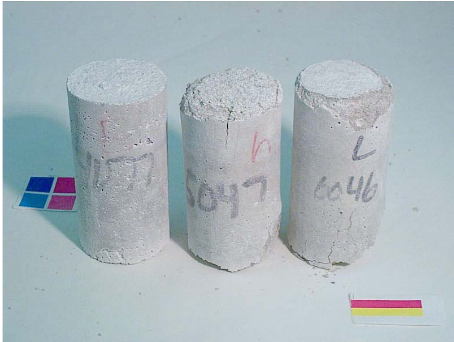
Figure 3.45 Cylinders exposed to \text{CaCl}_2 solution after 56 days of cyclic temperature test. From left to right: 0.40, 0.50, and 0.60 w/c mortar cylinders.
