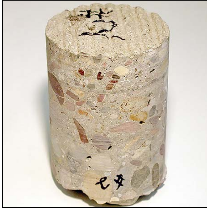
Figure 3.15. Core as received from Montana site, with little surface wear (MT_02).
