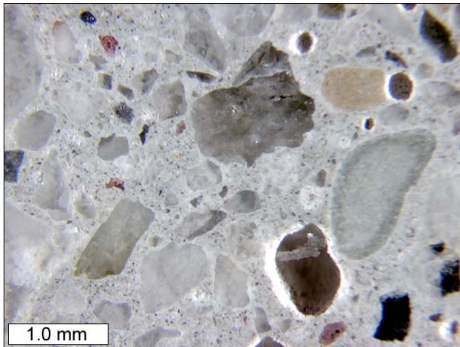
Figure 3.18. Stereomicroscope image of polished surface from core MT_02, magnified here approximately 22x.
