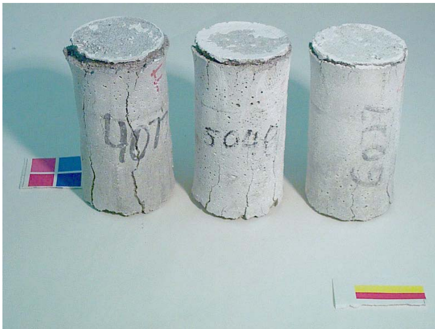
Figure 3.70. Cylinders exposed to CaCl_2 solution after 84 days of constant low temperature test. From left to right: 0.40, 0.50, and 0.60 w/c mortar cylinders.
