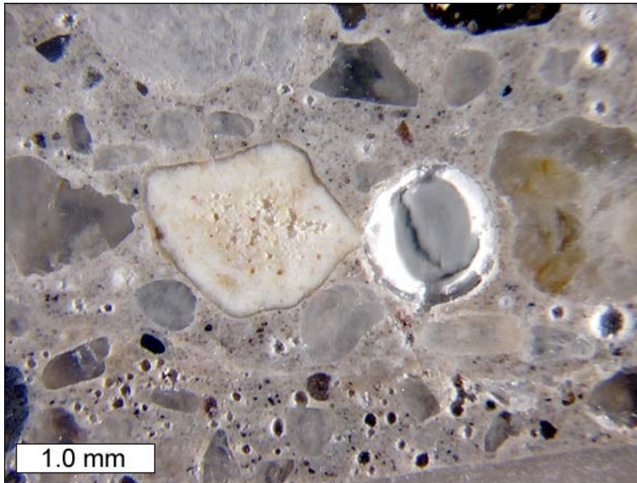
Figure 3.12. Stereomicroscope image of polished surface from core IA_07 showing alkali-silica reactive sand particle before staining procedure.
