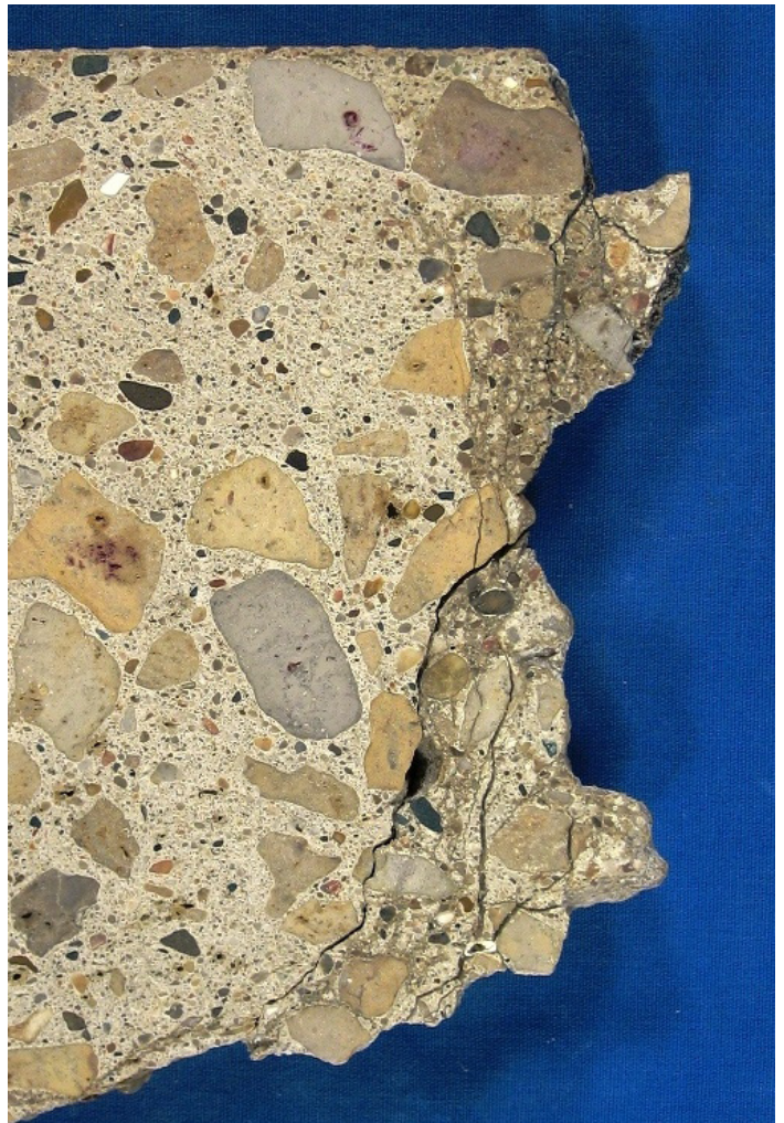
Figure 23. Deterioration due to bottom-up moisture
