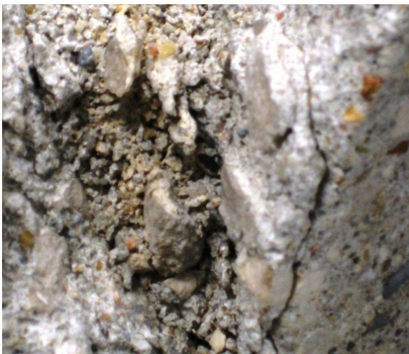
Figure 1. Typical slivers from freezing and thawing cycles
