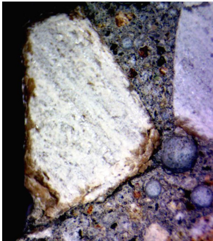
Figure 15. Photograph of an aggregate particle dislodged by inappropriate sawing (Field of view 5mm)
