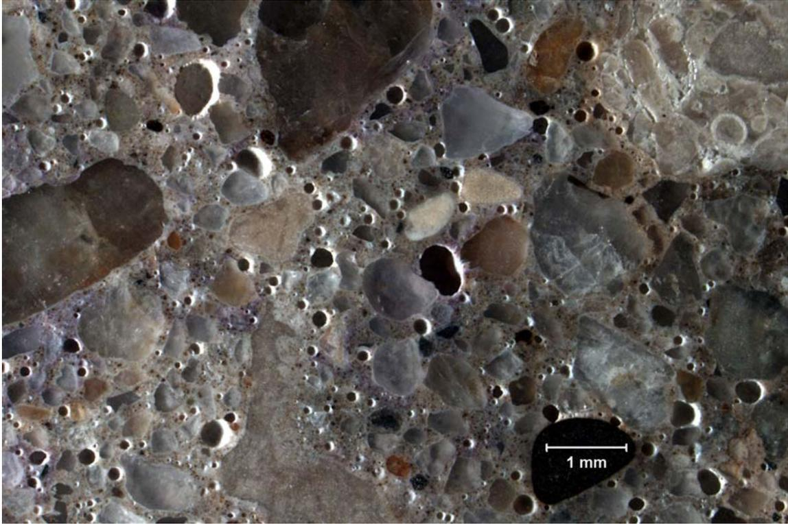
SAMPLE ID: #1 DESCRIPTION: Overall hardened air void content proximate to the top surface.
