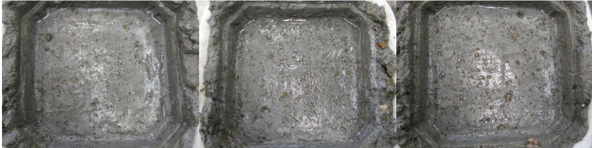
Figure 24. CA salt scaling sample after 50th freeze-thaw cycle
