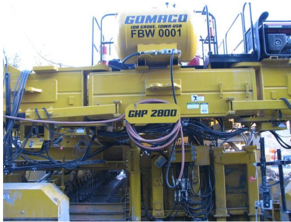
Figure 9. GOMACO GHP 2800 slipform concrete paver
