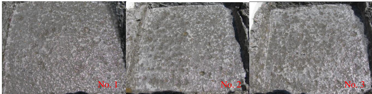
Figure 15. New York salt scaling specimens after 50th freeze-thaw cycle
