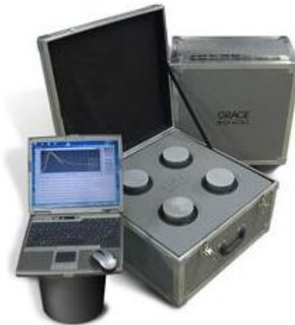
Figure 15. Adiacal calorimetry test equipment for heat of hydration of concrete
