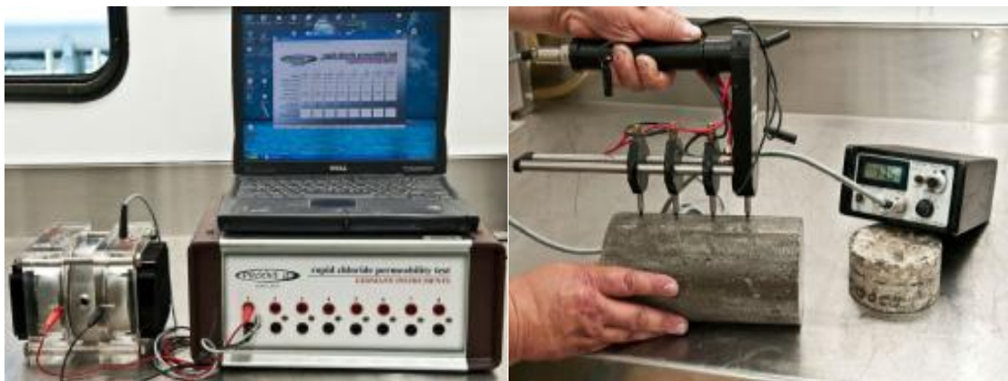
Figure 17. Rapid chloride permeability test (left) and surface resistivity meter (right)
