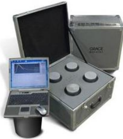
Figure 22. AdiaCal calorimetry test equipment for heat of hydration of concrete
