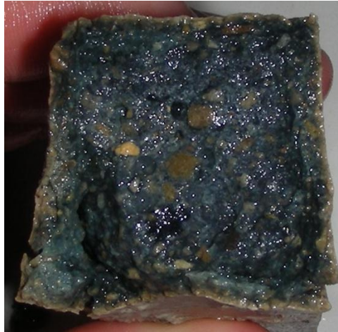
Figure 3. Internal sulfate attack damage
