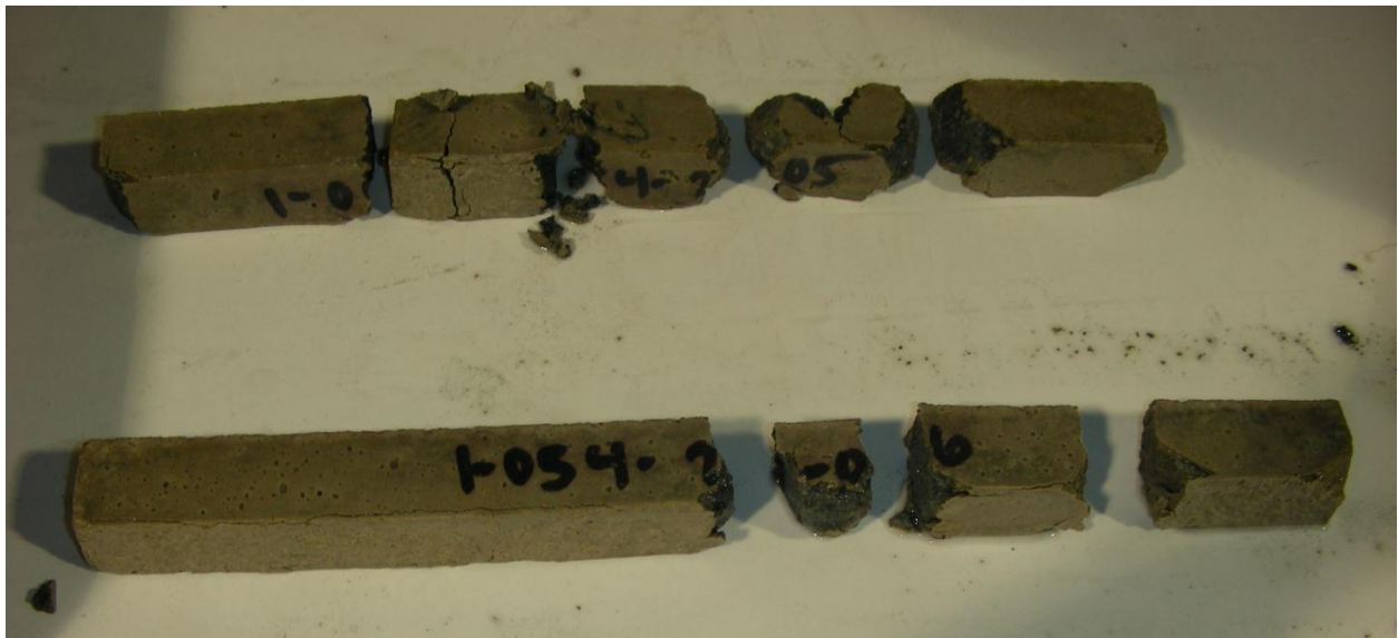
Figure 4. Severe sulfate damage
