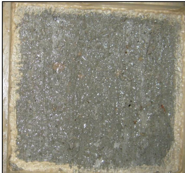
Figure 44. Visual rating of 2 (slight to moderate scaling)
