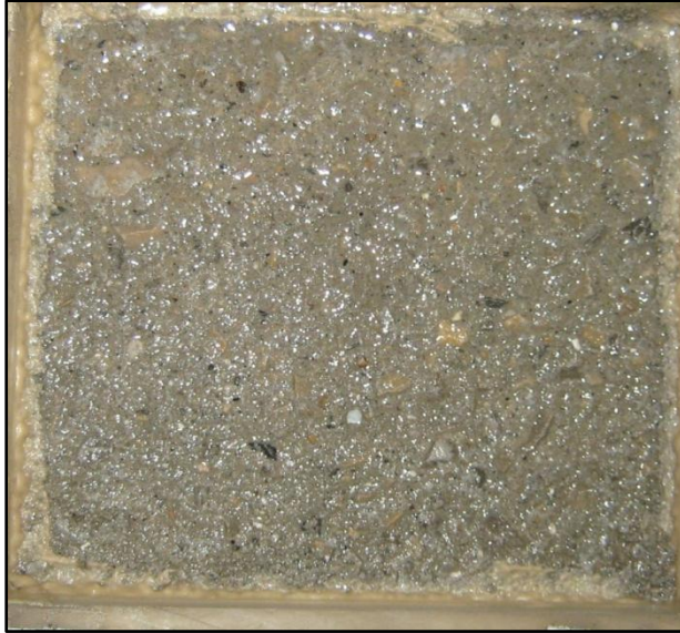
Figure 45. Visual rating of 3 (moderate scaling, some coarse aggregate visible)
