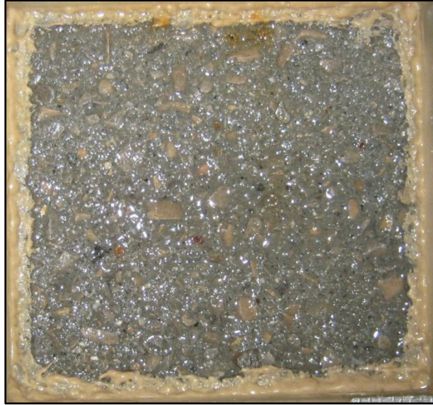
Figure 47. Visual rating of 5 (severe scaling, coarse aggregate visible over entire surface) scaling results
