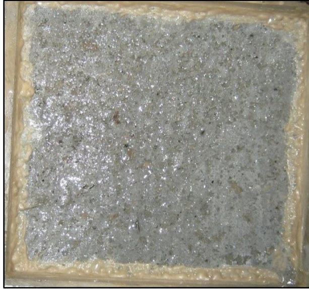
Figure 43. Visual rating of 1 (very slight scaling, 3 mm depth maximum, no coarse aggregate visible)
