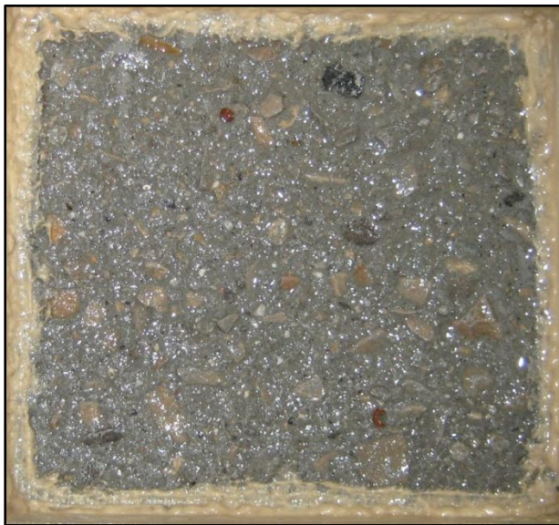
Figure 46. Visual rating of 4 (moderate to severe scaling)
