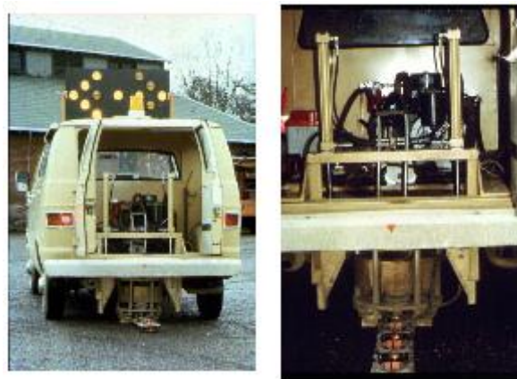
Figure 2.10. Road Rater (Muench et. al., 2005)
