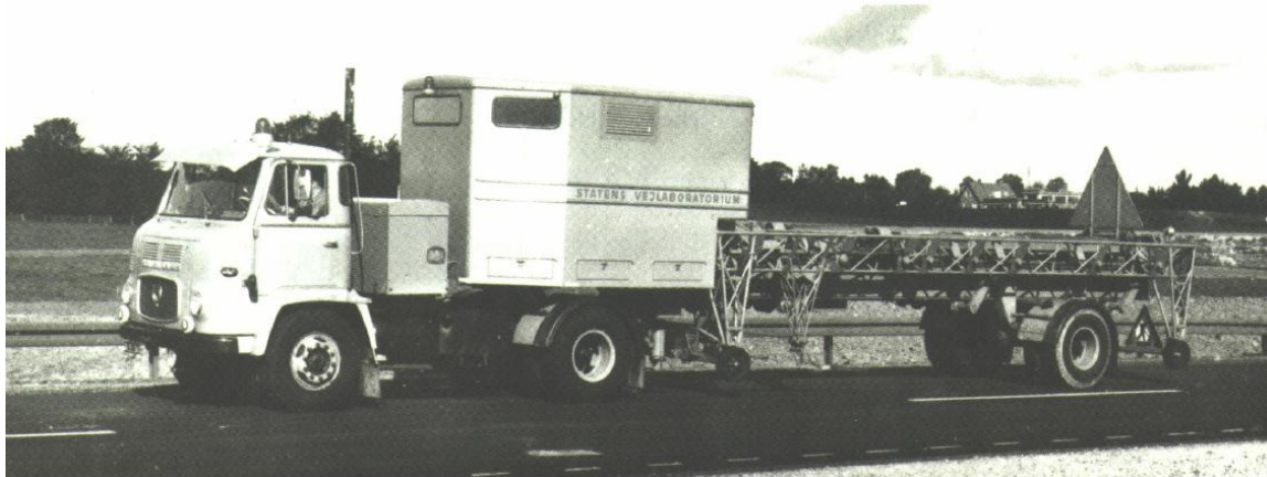
Figure 2.4. The Danish first generation Deflectograph (Christensen, 2003)
