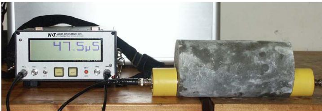
Figure 2.17. Typical ultrasonic test procedure (Ferraro 2003)
