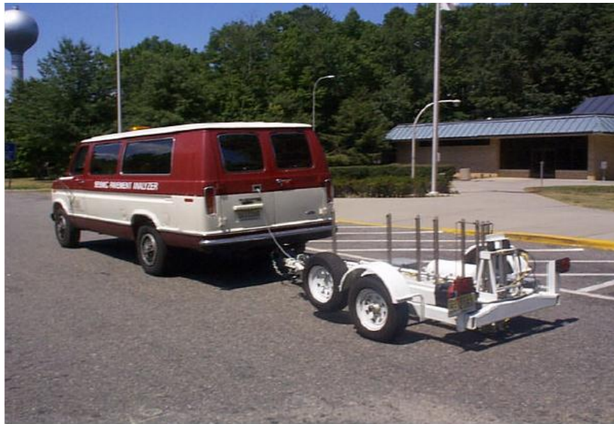
Figure 2.20. Seismic Pavement Analyzer (SPA)(Gucunski and Maher 2002)
