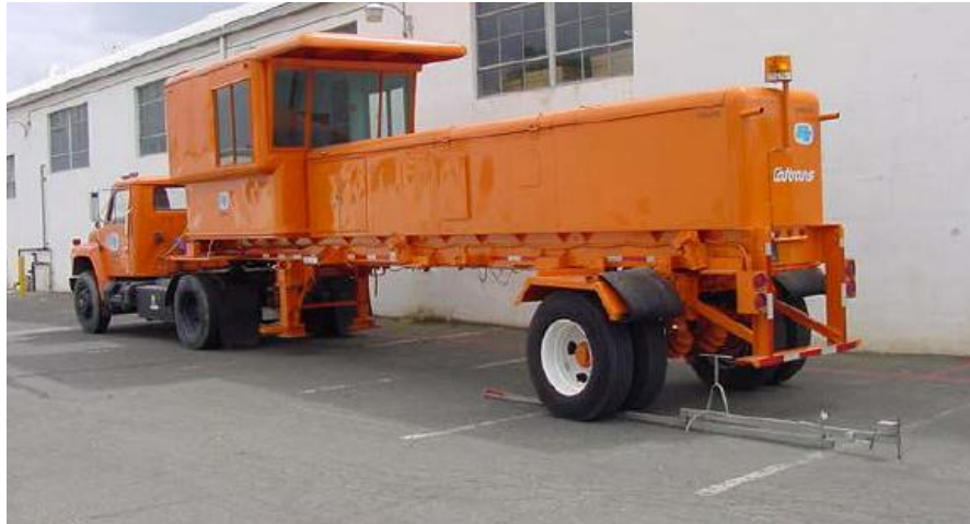
Figure 2.3. California traveling Deflectometer (Andren, 2006)
