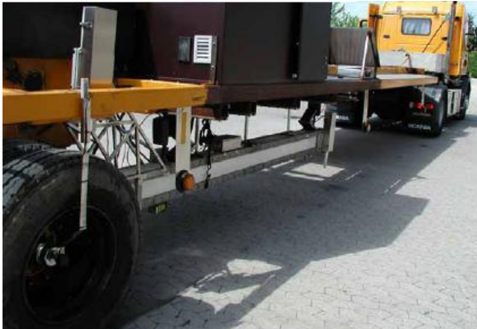
Figure 2.13. Prototype of High-Speed Deflectograph (HSD) (Hilderbrand, 2002)
