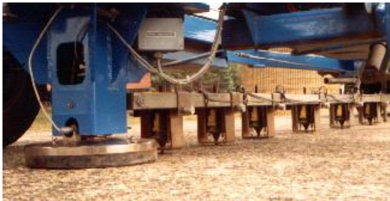
Figure 2.8. FWD bottom view with sensor locations (Muench et al., 2005)
