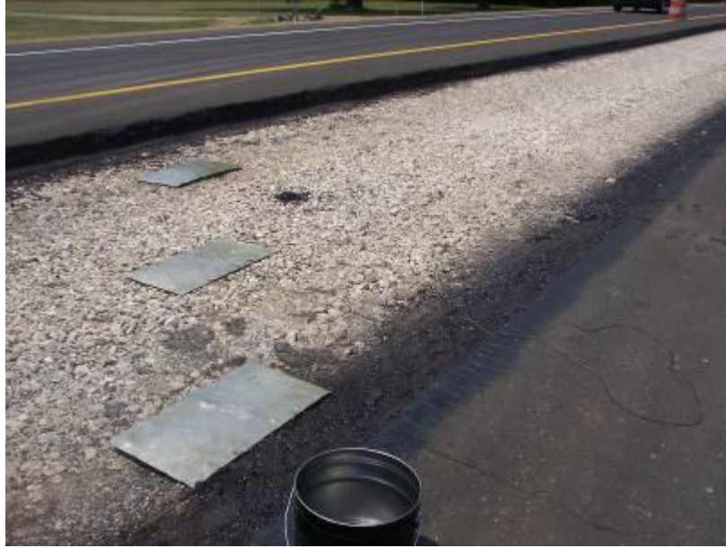
Figure 5-19 Plates randomly placed under HMA mat
