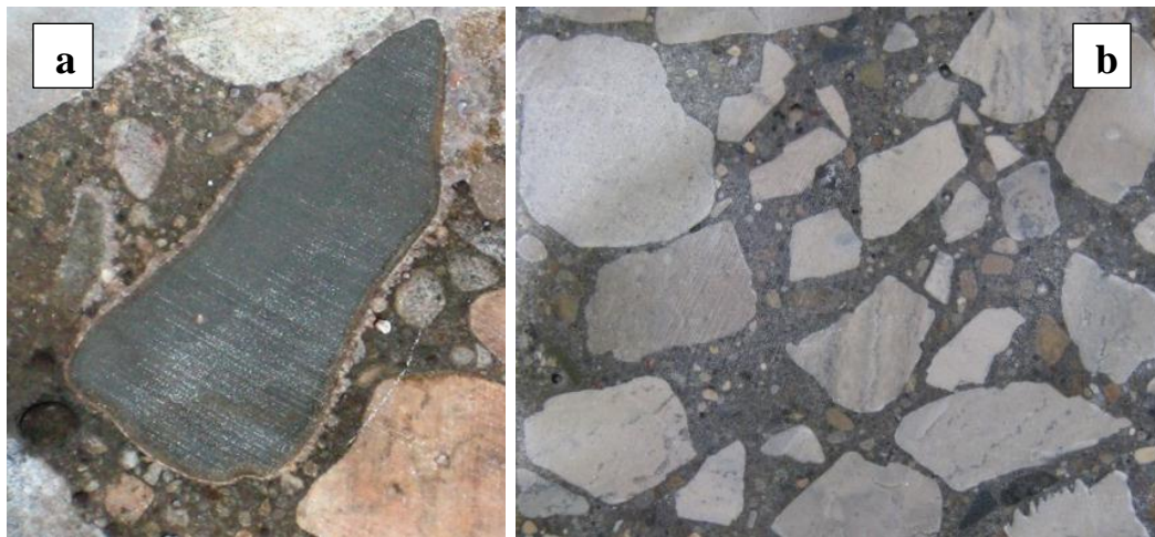
Figure 6. Silver nitrate sprayed samples for mapping chloride (a: concrete mixture using gravel; b: concrete mixture using limestone)
