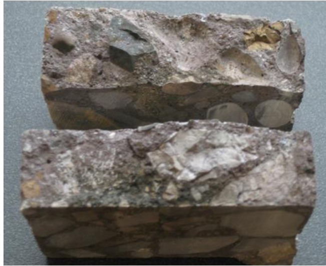
Figure 7. Fracture surface of silver nitrate sprayed samples
