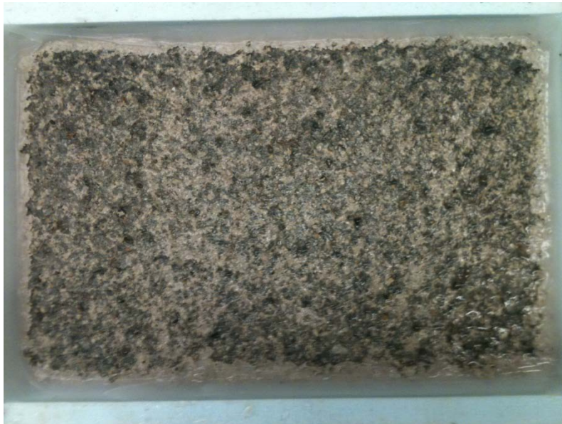
Figure 4. BNQ (VADOT curing) exposure for Mix #13 50%LA 50%SG120 0.42w/c at 25 cycles where finer sized pieces of scale were observed
